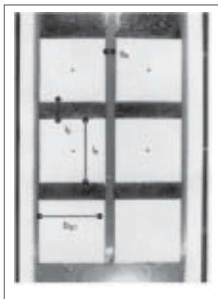
»6 Block setting in the water channel [2]
