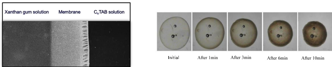
Figure 1. Left) polymer-surfactant membrane. Right) capsule shrinkage with time.
