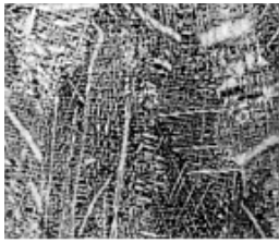
Fig. 19 Copper alloy 71500 (Cu-30Ni) ingot. Dendritic structure shows coring: light areas are nickel-rich; dark areas are low in nickel. 20 \times . 2
