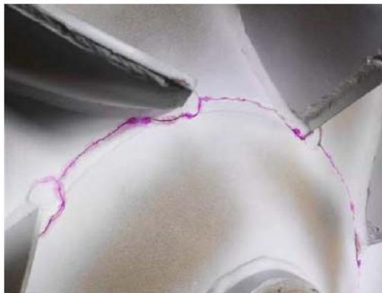
*Dye penetration in the stiffening cone of a turbine.*
