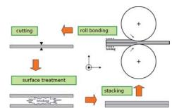
Fig. 2: Principle of Accumulative Roll Bonding
