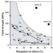
Fig.1: Cold rolling of Cu and Al increases the yield strength but decreases the elongation to failure (ductility) [1]
