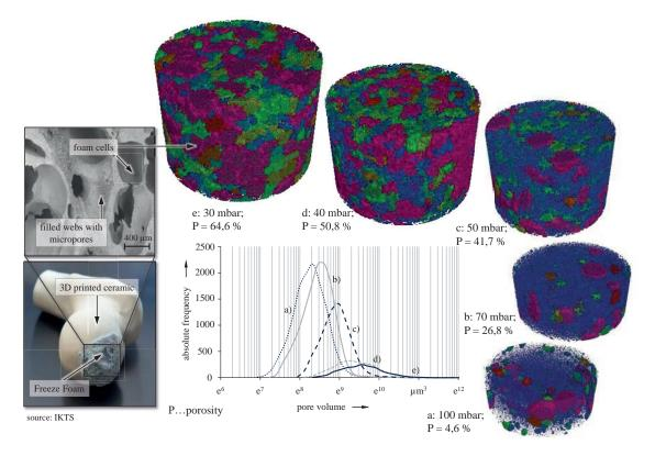
Pore size distribution during the foaming process at different pressure levels
