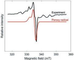
Simulated EPR spectra of peroxy radicals (20,7 %) in comparison to the experimental EPR spectrum of irradiated PVDF
