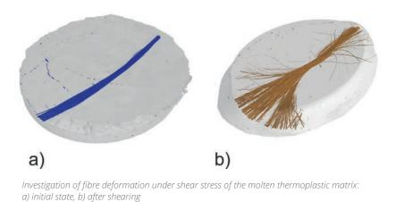
Fluid-structure interaction studies for the prediction of fibre displacement behaviour using the example of a large number of flexible structures in a fluid stream
