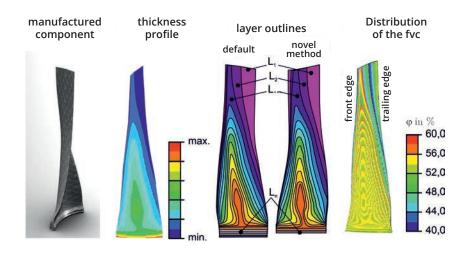
deficiencies of existing approaches are specifically addressed and remedied. In particular, the fibre volume content, which is the key parameter of every FRP component, plays a central role in the the method that has been developed.
