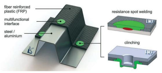
Multifunctional interfaces for joining FRP and metals using established spot joining technologies
