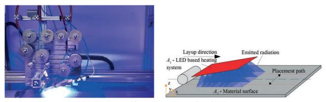
Laboratory placement unit with LED-based heating system (left), irradiation and heat transfer model (right)
