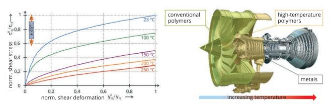
Measurement results from the tensile test on 45° laminates at different temperatures (left) for the design of turbine components (right)
