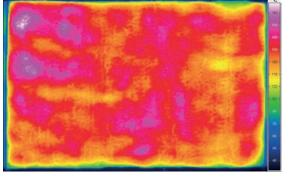
Thermographic image of a rCF nonwoven with a surface weight of 100g/m<sup>2</sup>
