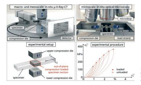
Fig. 2: Experimental procedure for cross-scale in-situ structure investigation under transverse pressure loading
