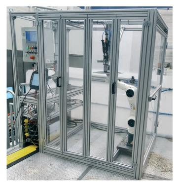
Automated manufacturing cell for 3D-printing of thermoset continuous fibre reinforced composite parts
