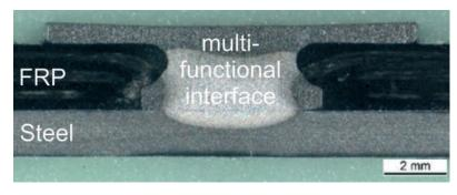
Micrograph of a welded joint with multifunctional interface © LWF
