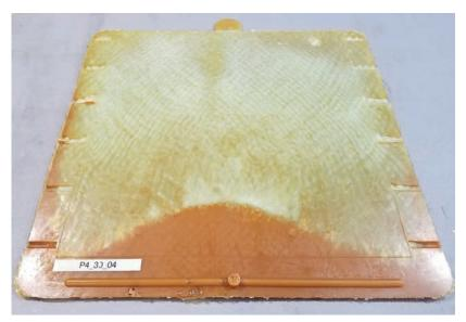
Test plate with conspicuous fibre misorientations and resin rich areas
