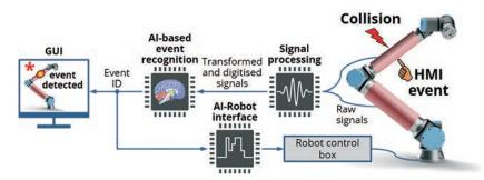
Schematic overview of the planned human-machine interaction with an intelligent sensor layer on robots
