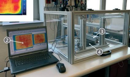
Experimental test stand for electrical characterization and thermographic images of rCF nonwovens
