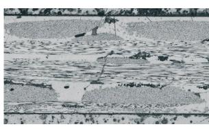
Micro-structure analysis of a glass-fibre (GF) reinforced epoxy resin
