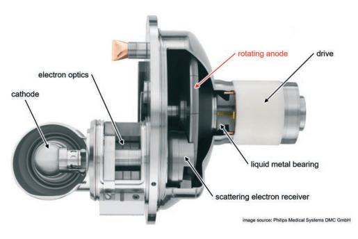
Sectional model of an X-ray tube to illustrate the setup with metallic rotating anode
