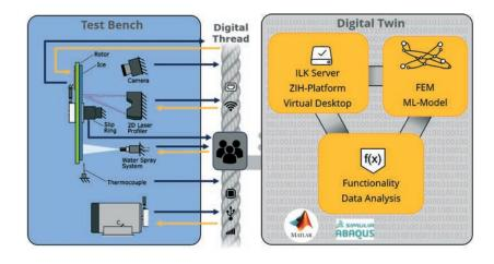
*IVeT architecture shown on the example of an rotor test bench connected to its digital twin via the digital thread*
