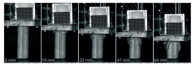
High speed camera recordings during drop-tower test of crash absorber sub-structure with drop height: 3.30 m, drop mass: 92.2 kg and crash absorber length: 140 mm
