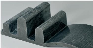
Prototypical demonstrator structure with complex geometry consisting of foam impregnated textile-reinforced cover layers and polyurethane core layer
