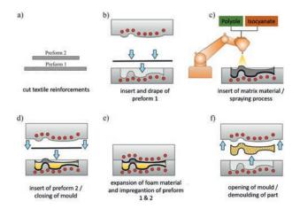
Schematic representation of the foam impregnation process
