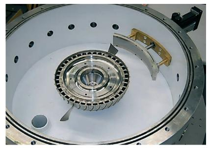
Fig. 1: Test chamber of the blade strip test rig
