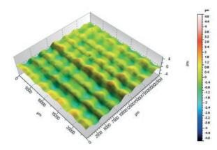
Topology of an GF-epoxy surface generated by 3D laserprofilometry
