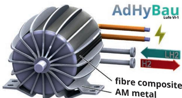
Generative manufacturing technologies enable optimized cooling systems and a specific coil design to increase the power density of next-generation electric motors.
