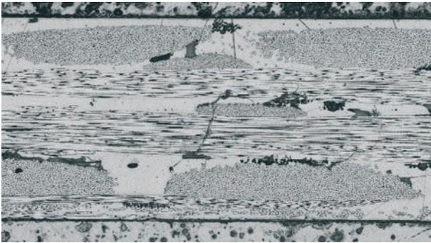
Micro-structure analysis of a glass-fibre (GF) reinforced epoxy resin
