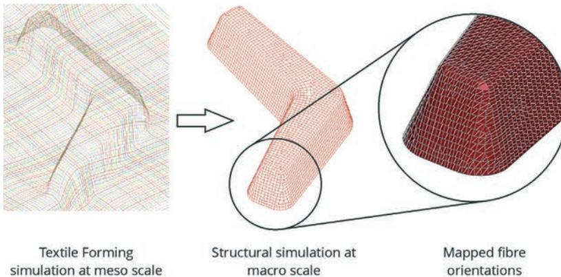
Textile Forming simulation at meso scale
