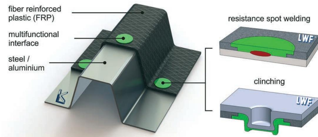
Multifunctional interfaces for joining FRP and metals using established spot joining technologies
