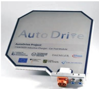
Laboratory demonstrator of the inductive charging system on vehicle side
