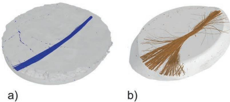
Investigation of fibre deformation under shear stress of the molten thermoplastic matrix:
