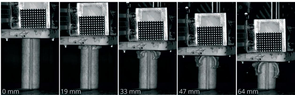
High speed camera recordings during drop-tower test of crash absorber sub-structure with drop height: 3.30m, drop mass: 92.2kg and crash absorber length: 140mm
