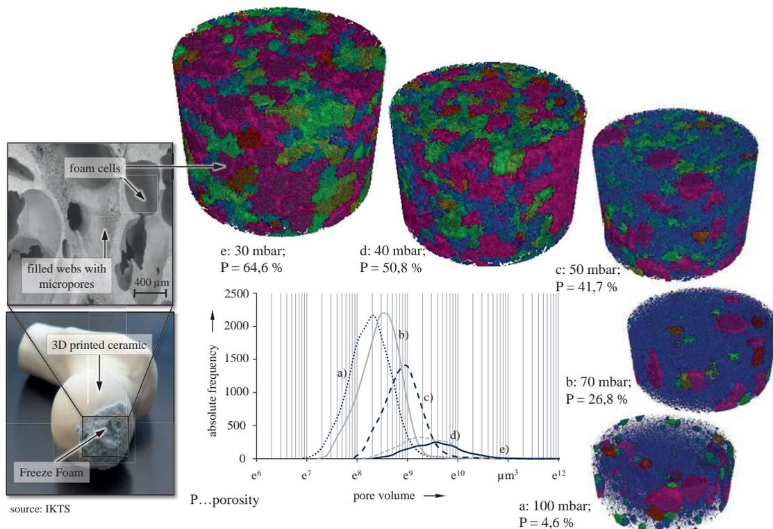
Pore size distribution during the foaming process at different pressure levels
