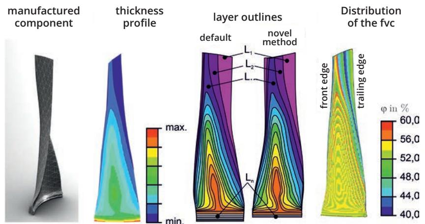
deficiencies of existing approaches are specifically addressed and remedied. In particular, the fibre volume content, which is the key parameter of every FRP component, plays a central role in the the method that has been developed.
