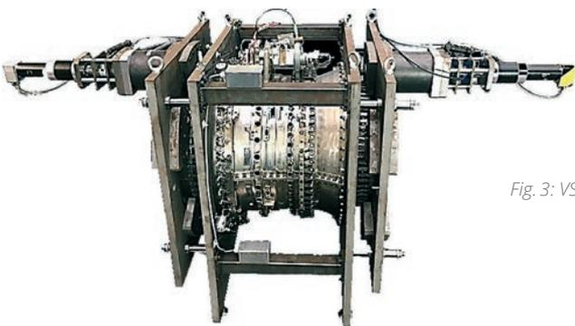
Fig. 3: VSV-multi stage test rig
