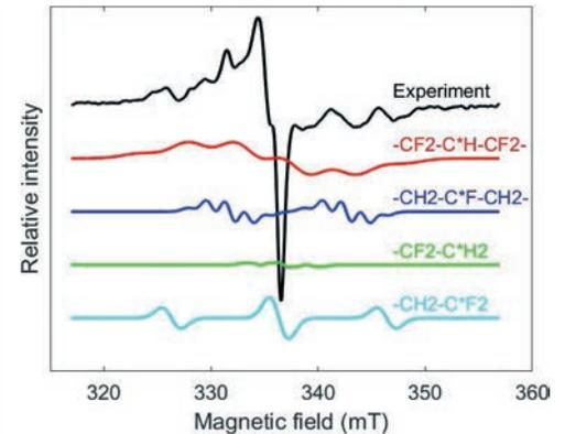
Simulated EPR spectra of alkyl radicals (74,4%) in comparison to the experimental EPR spectrum of irradiated PVDF
