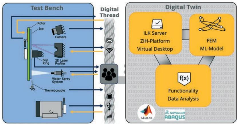
IVeT architecture shown on the example of a rotor test bench connected to its digital twin via the digital thread
