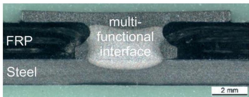
Micrograph of a welded joint with multifunctional interface
