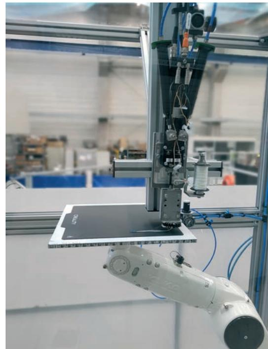
Print head for 3D printing of continuous fibre-reinforced polymers
