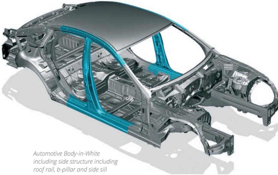
Automotive Body-in-White including side structure including roof rail, b-pillar and side sill
