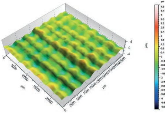
Topology of an GF-epoxy surface generated by 3D laserprofilometry
