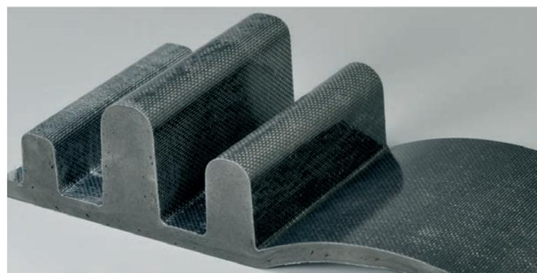
*Prototypical demonstrator structure with complex geometry consisting of foam impregnated textile-reinforced cover layers and polyurethane core layer*
