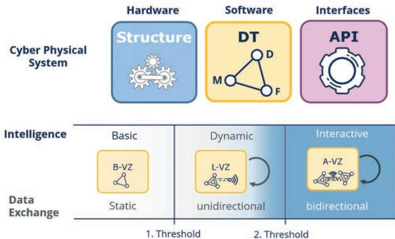
The three main development stages of a digital twin based on their data exchange capabilities
