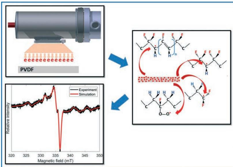
Overview on electron induced generation of radicals in PVDF and simulation of EPR spectra
