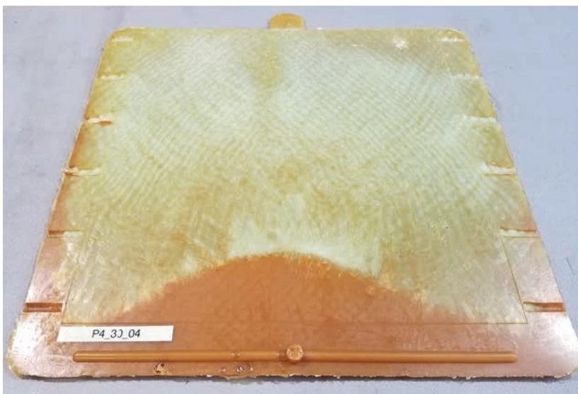
Test plate with conspicuous fibre misorientations and resin rich areas
