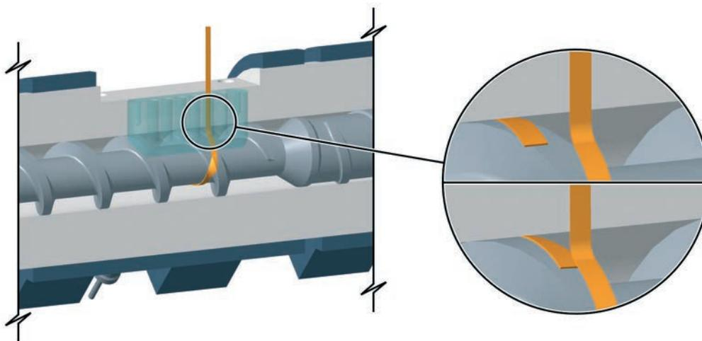
*Fibre conveying inside of an injection-molding plasticizing unit*
