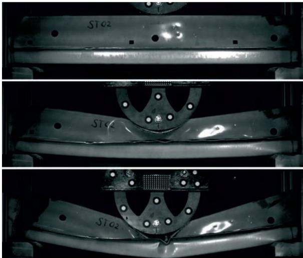
Drop tower crash test of reference steel side sill structure
