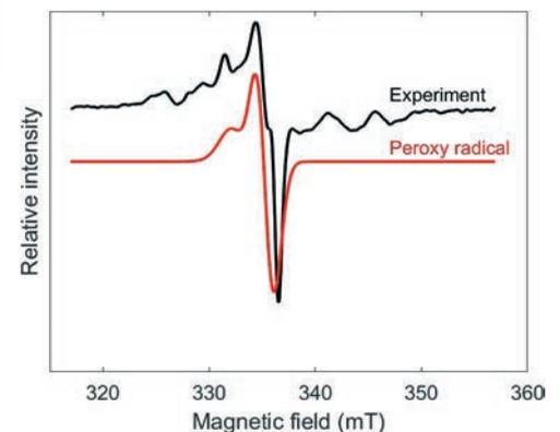
Simulated EPR spectra of peroxy radicals (20,7%) in comparison to the experimental EPR spectrum of irradiated PVDF
