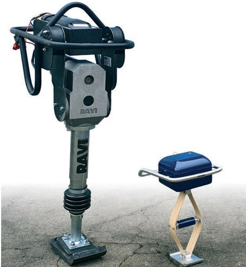
Electrically driven vibrating tamper (left) and demonstrator for a tamper utilizing a deltoid mechanism with compliant joints (right)
