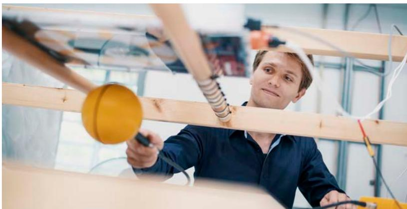
Measurement of the electromagnetic field of inductive charging systems on the HiL test bench of the ILK
