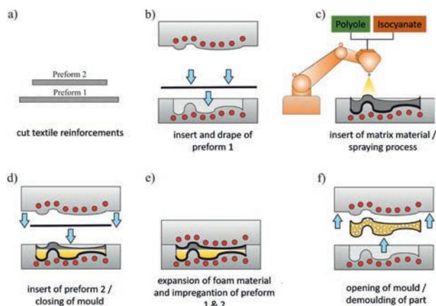
*Schematic representation of the foam impregnation process*
