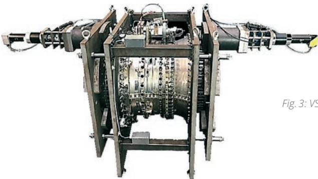
Fig. 3: VSV-multi stage test rig
