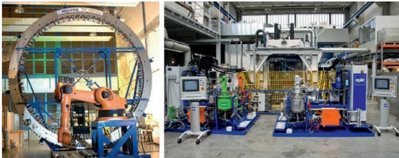
Radial braiding wheel (left) and HP-RTM infiltration system (right) from ILK are used to manufacture the test plates and structures
