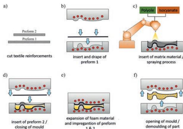
*Schematic representation of the foam impregnation process*
