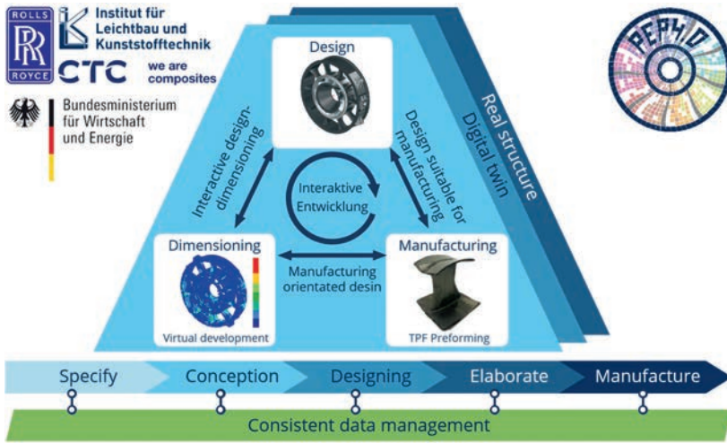
Fig. 1: Interactive development process with the individual disciplines of design, layout and manufacturing (top) along the phases from specification of requirements to manufacturing (bottom)
