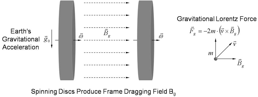
Figure 1: Principle of Generating a Lorentz-Type Acceleration using Frame-Dragging-Like Fields
