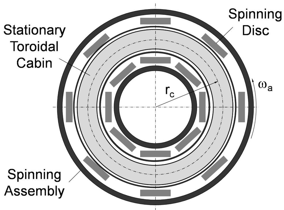
Figure 3: Circular Artificial Gravity Generator using Spinning Discs
