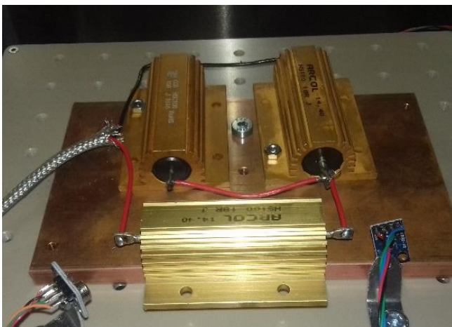
Figure 22: Resistor Setup on Copper Plate (left), Average Resistor – 0°, Sine, 75 V, 9.6 kHz
