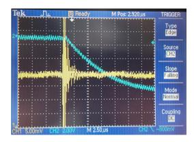
Figure 5. Induced EMP picked up by our oscilloscope. Channel 1 (5 mV/div) is measuring the output of an accelerometer, while Channel 2 (2 V/div) is measuring the output from the current sensor
