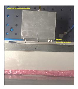
Figure 14. The optical accelerometer (topcenter) facing the cryostat and the piezoaccelerometer (top-right) placed vertically for the reference measurements of the EMP influence
