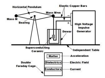
Figure 2. Schematic of Poher's Experimental setup and sensor arrangement<sup>11</sup>
