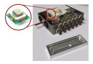
Figure 6. Accelerometer and Hall sensor assembly without the top cover
