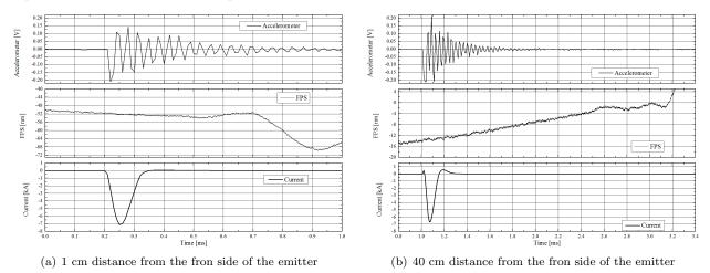
Figure 15. Representative measurements done with the optical accelerometer and piezo-accelerometer during discharges of 2.2 kV
