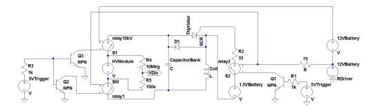
Figure 4. Schematic of the small-scale impulse generator's circuit
