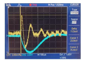
Figure 10. Anomalous accelerometer readout during a 500 V DC discharge through an YBCO disc below its critical temperature. CH1 is the accelerometer output (1.2 V/g) and CH2 is the current output (1 V/1 kA)
