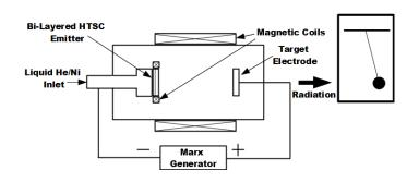
Figure 1. Schematic of Podkletnov's experimental setup<sup>1</sup>
