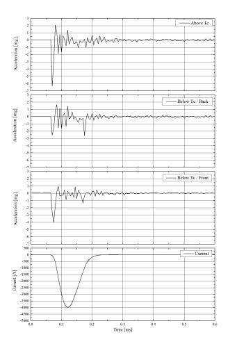
Figure 13. Measurement results with the piezoelectric sensor during discharges of 1.2 kV into the 22 mm YBCO disc
