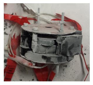
Figure 16. Destroyed support and superconductors by the double HTSC disc configuration during 1.7 kV discharges (photo taken right after the assembly was dismounted from the cryostat)
