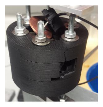
Figure 12. The destroyed second support after a few discharges at 1.3 kV into the YBCO disc
