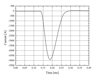
Figure 11. Current impulse profile of a 1.7 kV discharge into a 22 diameter, 3 mm thick aluminum disc at room temperature
