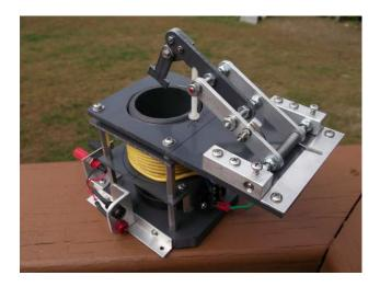
Figure 3. Schroeder's coil and HTSC disc support assembly<sup>4</sup>
