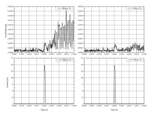
Figure 8. Magnitude of the 3-D acceleration field change measured during 20 impulses and averaged in non-superconducting (right) and superconducting state (left) of the YBCO disc
