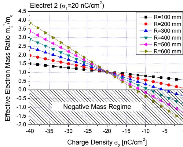
Figure 6. Effective Electron Mass Ratio Dependence on Disc Radius and Charge Density  $\sigma_2$ .
