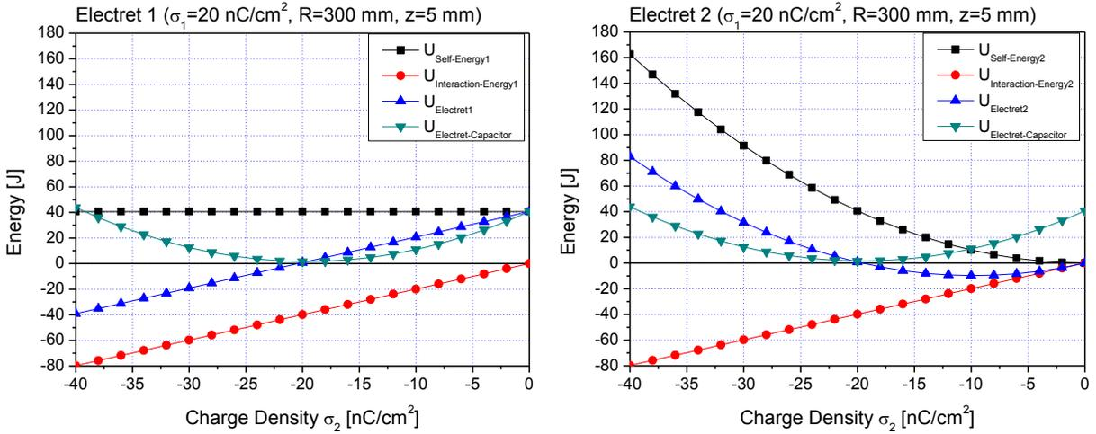
Figure 5. Dependence of Electret Plates Energy on Charge Density  $\sigma_2$ .
