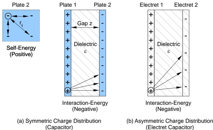
**Figure 4. Self- and Interaction-Energy Contribution to the Total Energy Stored in a Capacitor or Electret-Capacitor.**
