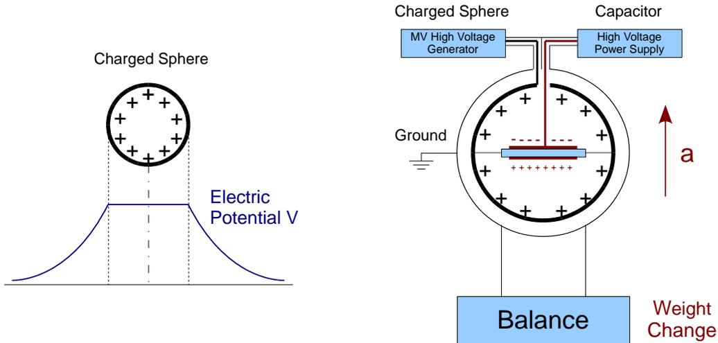
Figure 3. Self-Acceleration of a Capacitor inside a Positively Charged Dielectric Shell.
