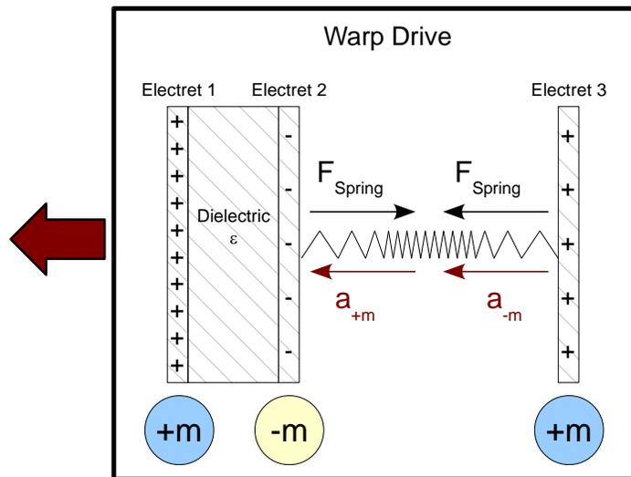
**Figure 7. Space Drive Concept based on 3-Plate Electret Capacitor.**
