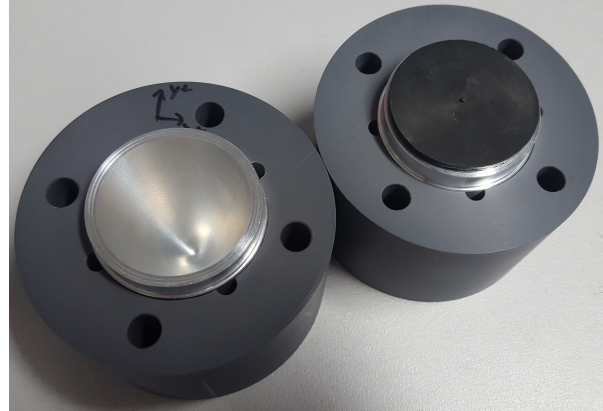
Figure 10. The paraboloid electrodes inside their polyamide insulation with the 45 mm diameter single-crystal YBCO superconductor disc (right). The small seed crystal can be seen in the middle of the disc.
