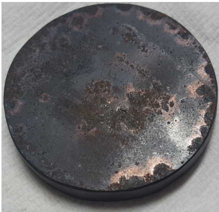
Figure 14. The eroded surface of the sintered superconductor disc, through which numerous impulses were performed in air and LN2
