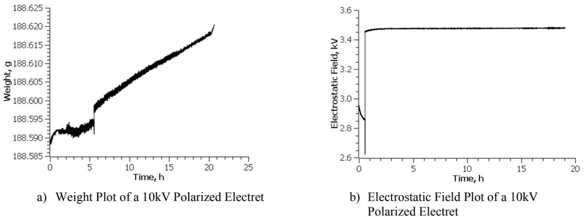
**Figure 7. Characteristics of Polarized Polycarbonate Container Electrets.**
