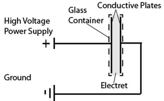
Figure 11. Schematic View of the Electret Polarization with a Glass Container.
