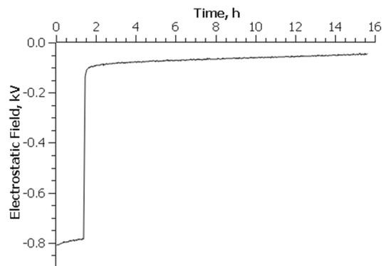
b) Electrostatic Field plot of a 10kV Polarized Electret, Measured on the Side where the Negative Electrode was Located
