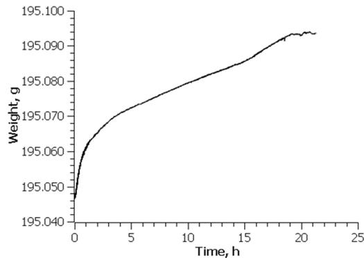
**Figure 9. Weight Plot of a Non-Polarized Polycarbonate Container Electret.**
