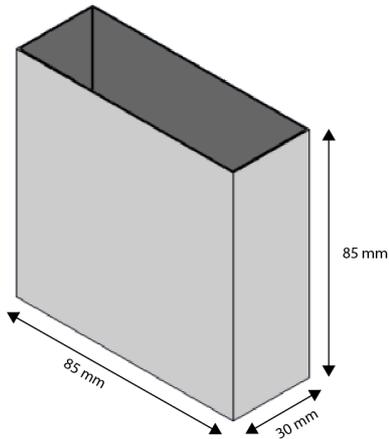
**Figure 4. Polycarbonate Container for Electrets.**
