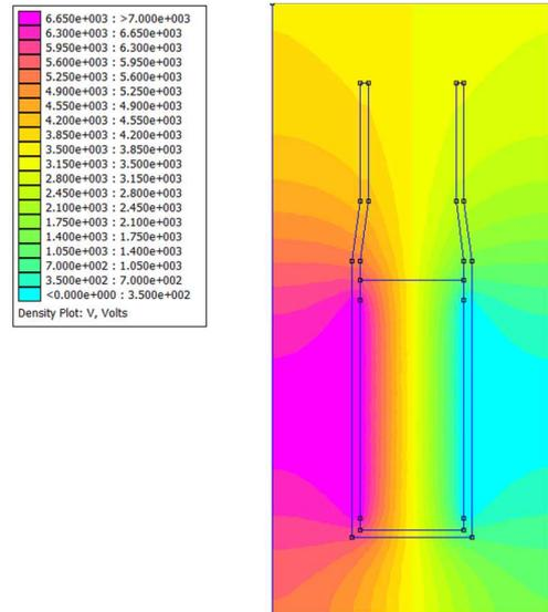
Figure 13. Contour of the Electrostatic Field Generated by the Electrodes inside a Glass Container Electret assuming a 7kV Polarization.
