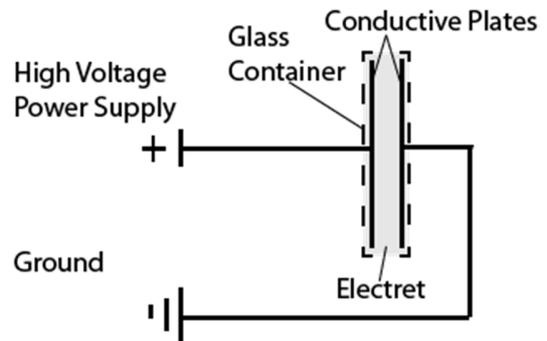
**Figure 11. Schematic View of the Electret Polarization with a Glass Container.**
