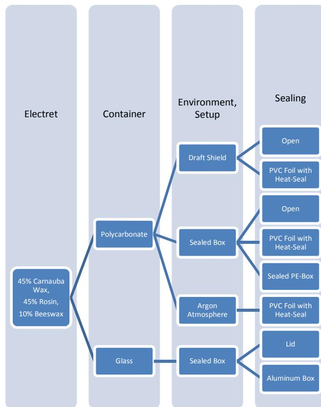
**Figure 1. Different Experimental Setups.**
