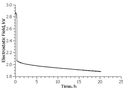
a) Electrostatic Field Plot of a 10kV Polarized electret, Measured on the Side where the Negative Electrode was Located
