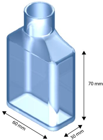
**Figure 10. Glass Container for Electrets.**
