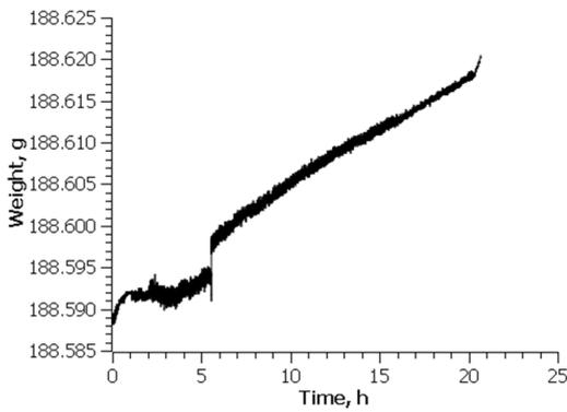
a) Weight Plot of a 10kV Polarized Electret
