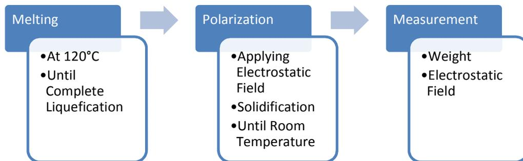
**Figure 2. Procedure of Electret Manufacturing.**
