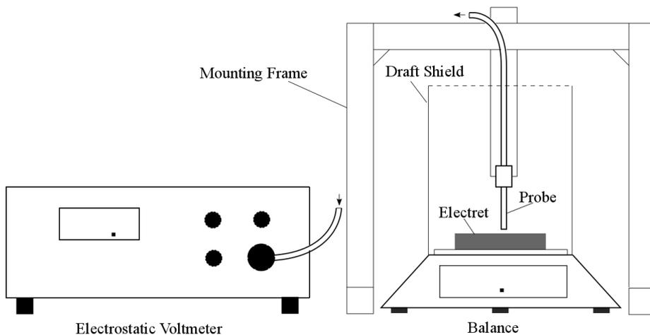
**Figure 6. Schematic View of the Measurement Setup for Polycarbonate Container Electrets.**
