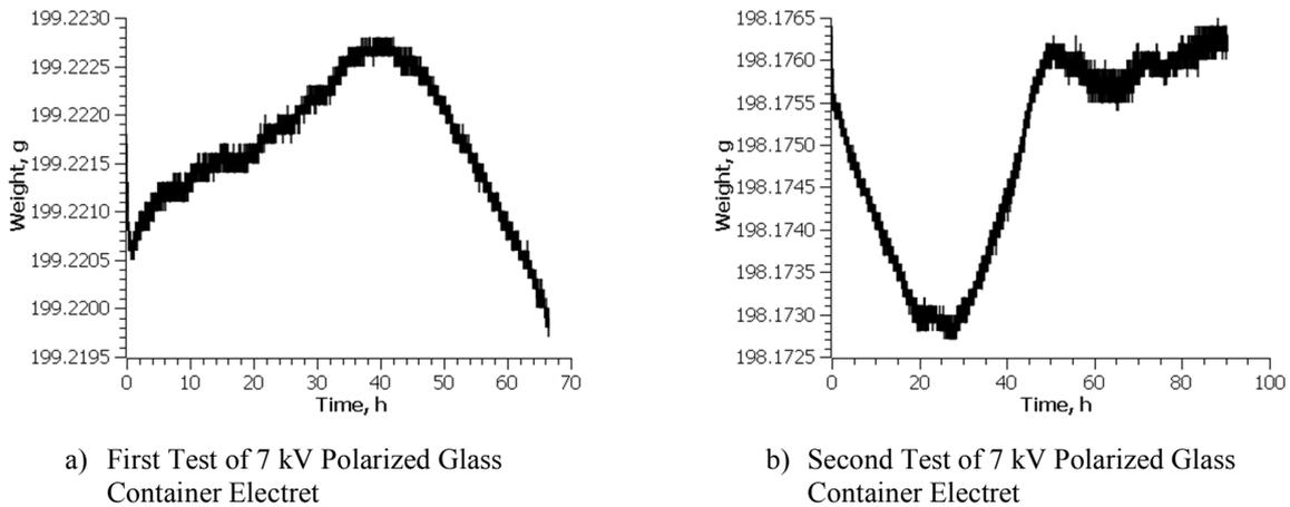
**Figure 14. Weight Plot of Polarized Glass Container Electrets.**
