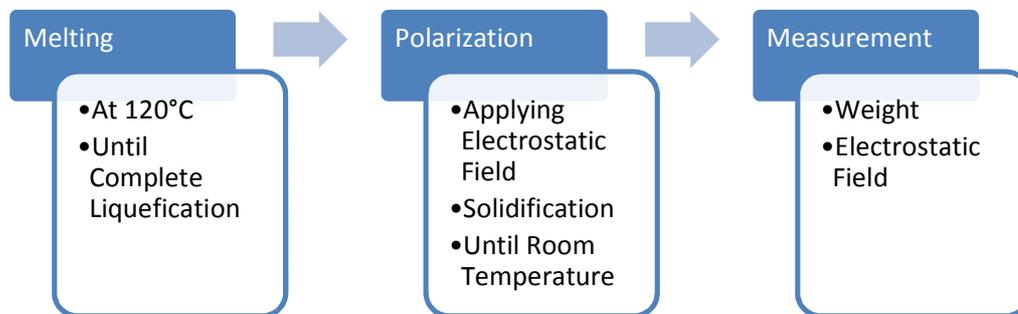
**Figure 2. Procedure of Electret Manufacturing.**
