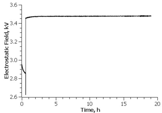
b) Electrostatic Field Plot of a 10kV Polarized Electret
