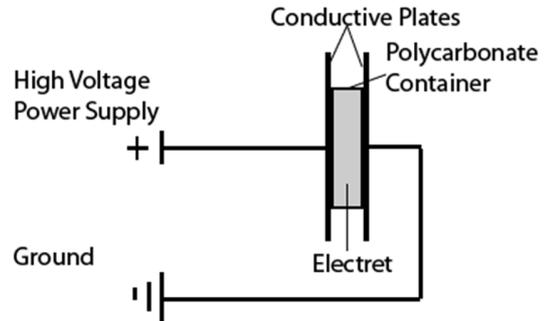
**Figure 5. Schematic View of the Electret Polarization with a Polycarbonate Container.**
