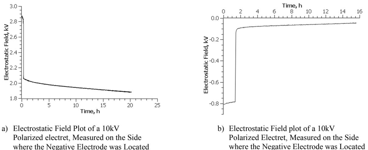
**Figure 8. Electrostatic Field Plot of Polarized Electrets.**
