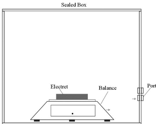
Figure 12. Schematic View of the Weight Measurement Setup for Glass Container Electrets
