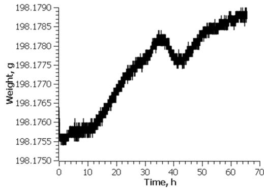
**Figure 15. Weight Plot of a Non-Polarized Glass Container Electret.**
