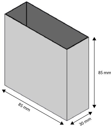
**Figure 4. Polycarbonate Container for Electrets.**
