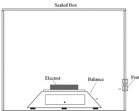
**Figure 12. Schematic View of the Weight Measurement Setup for Glass Container Electrets**
