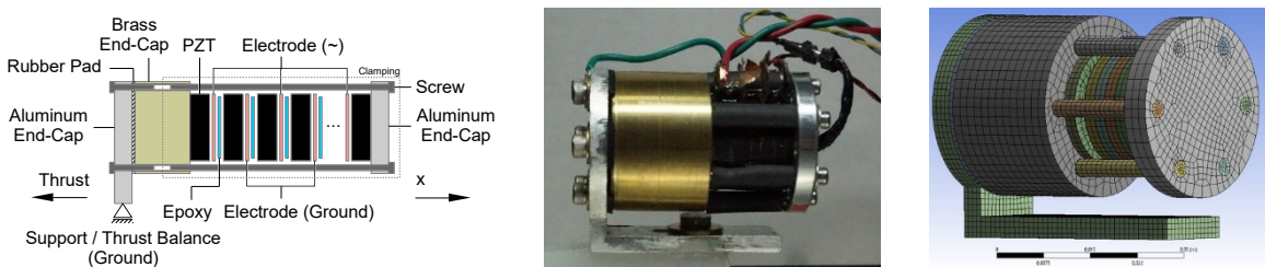
Fig. 11 Mach-Effect Thruster (MET): Schematic Sketch (Left) [24], Thruster under Testing (Middle) and ANSYS Model (Right)
