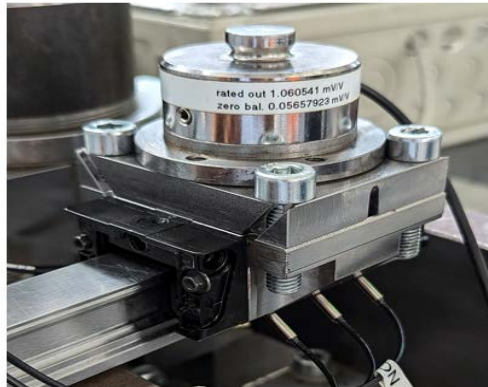
Fig. 1: Profile Rail Guide with Integrated Sensors
