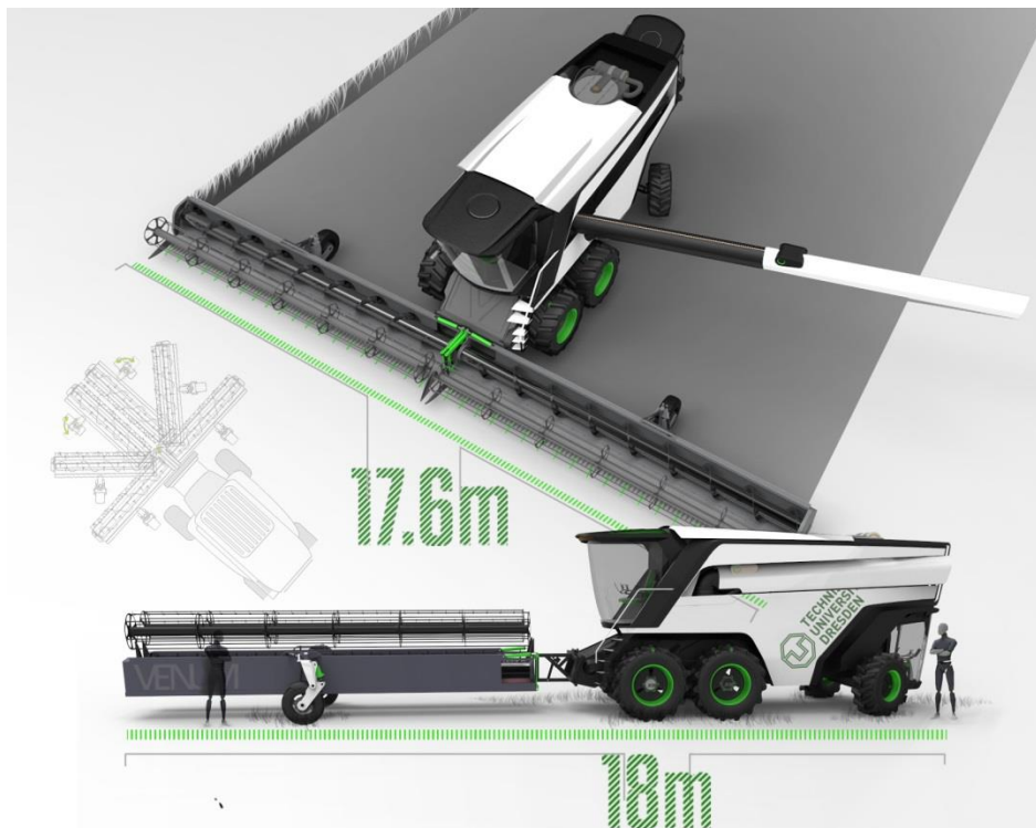
Fig. 2: The VENUM in harvest and transport configuration
