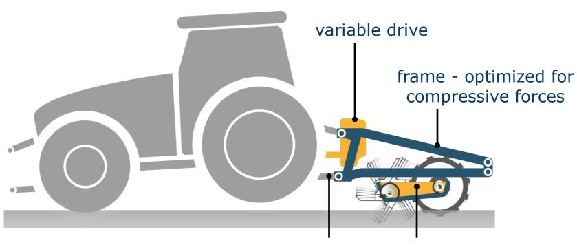
kinematic to lift up rear axle from tractor
