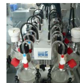
RAMOS including 8 shaking flasks for measurement, each with suspension of H. annuus
