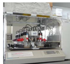
RAMOS including 8 shaking flasks for measurement, each with suspension of H. annuus
