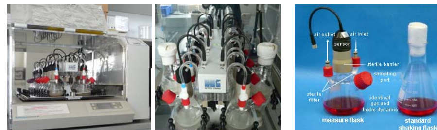
RAMOS ® including 8 shaking flasks for measurement, each with suspension of H. annuus
