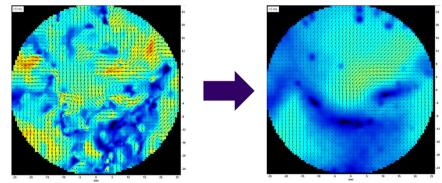
POD filtered PIV data to identify in-cylinder swirl structures
