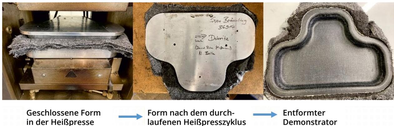
Abb. 7: Umformprozess zur Herstellung des 3D-rCFRP-Demonstrators „T-Napf“ / Forming process for the realization of the 3D-rCFRP demonstrator "T-cup"
