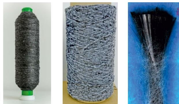
Abb. 3: Verschiedene Garnkonstruktionen aus rCF / Different yarn constructions consisting of rCF (realized by roving frame, wrap and friction spinning)
