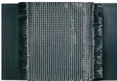
MLG-Patch (li.) zur Reparatur von CFK-Bauteilen (re.) / MLG patch (l.) for the repair of CFRP components (r.)
