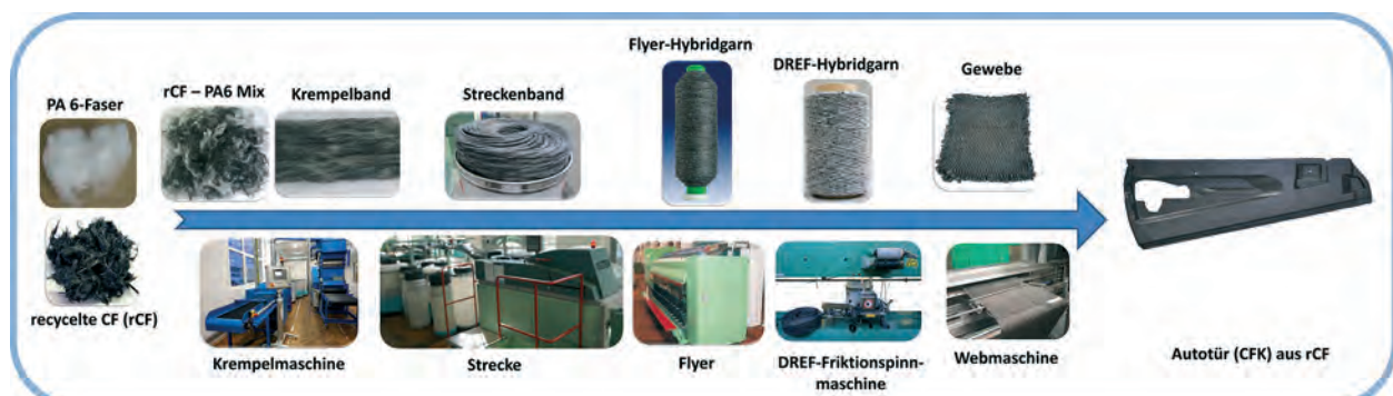
Abb. 1: Am ITM entwickelte Prozesskette zur Herstellung von rCF-Composites / Process chain for the manufacturing of rCF composites developed at ITM
