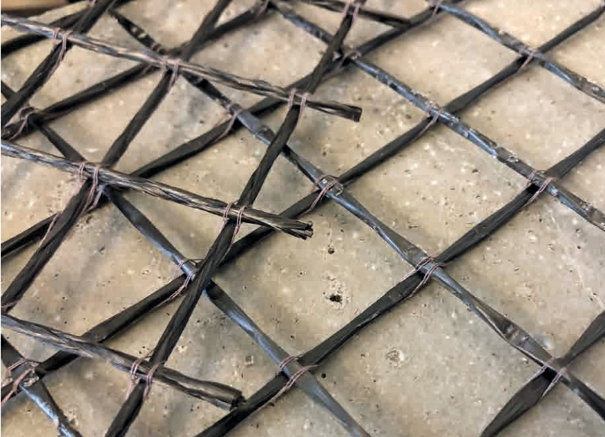
Abb. 5: Textilbetonbewehrung aus Flecht- (links) und Profilgar- nen (rechts) / Carbon concrete reinforcement structure made of braided (left) and profiled yarns (right)
