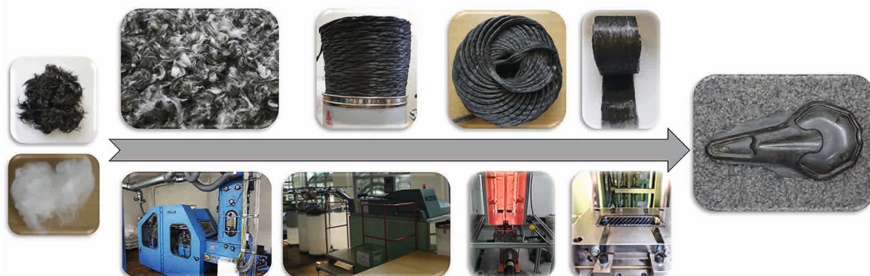
Abb. 1: Am ITM entwickelte Prozesskette zur Herstellung von rCF-Composites / Process chain for the manufacturing of rCF composites developed at ITM
