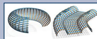
In the category, "New Processing Techniques," the ITM received the highly-esteemed Techtextil Innovation Award 2009 for its development of "Three Dimensional Laid Scrims." Highlighted was the development of the innovative processing technology known as an individual warp thread feed, which makes possible the manufacture of planar and spatially curved textile structures with load-oriented reinforcing threads.
