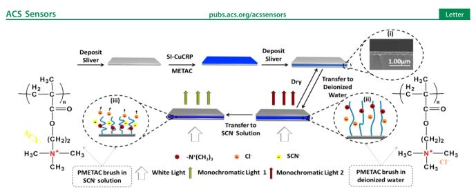
Figure 1. Schematic diagram of the preparation process and the detection principle of the as-prepared MIM resonator. Insets show the crosssectional SEM image of the MIM resonator (i) and the conformation of PMETAC chain in deionized water (ii) and electrolyte solution (iii).
