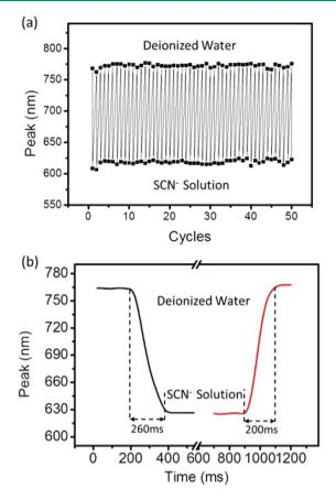
Figure 4. (a) Detecting cycles of the resonator between deionized water and  $SCN^-$  solution. (b) Peak position against time of the asprepared MIM resonator as the external environment changes.
