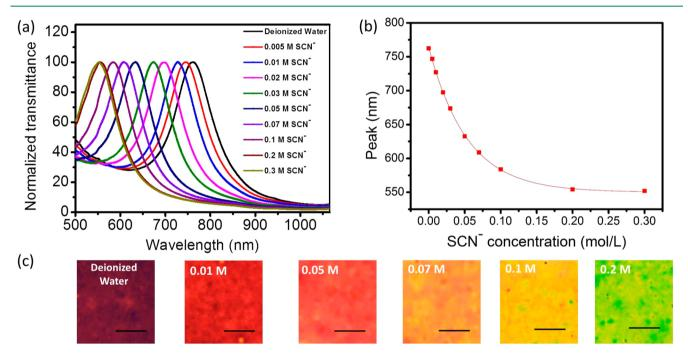
Figure 2. (a) Transmittance spectra of the as-prepared MIM resonator in different solutions. (b) Relation curve between the shift of the peak and the concentration of the SCN<sup>-</sup> solutions. (c) Optical photographs of the as-prepared MIM resonator in different concentrations of SCN<sup>-</sup> solutions (the bar is 10  $\mu$ m).
