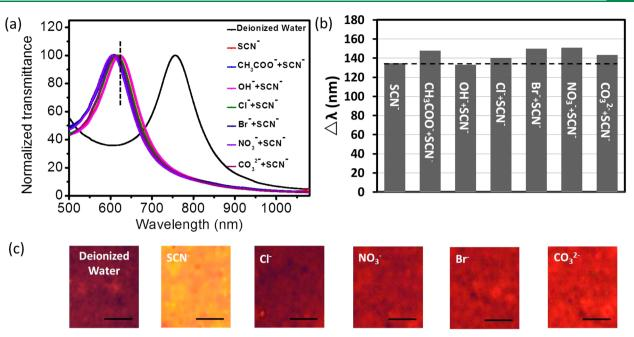
Figure 3. (a) Transmittance spectra of the as-prepared MIM resonator in water, SCN<sup>-</sup>, and mixtures of SCN<sup>-</sup> and disturbing anions. (b) {eak of the as-prepared MIM resonator for detecting SCN<sup>-</sup> in different solutions and water. (c) Photographs of the as-prepared MIM resonator in different anion solutions (the bar is 10  $\mu$ m).
