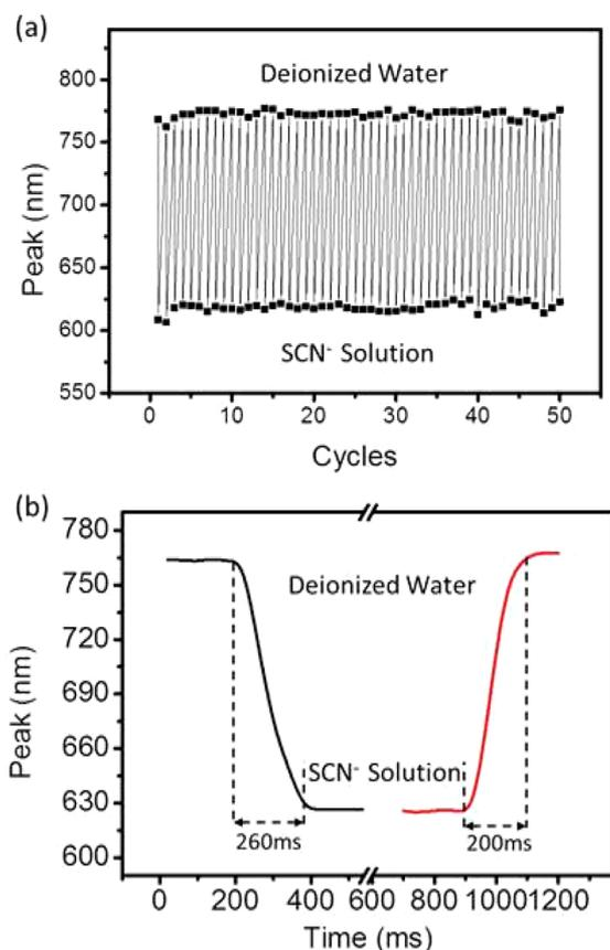
**Figure 4.** (a) Detecting cycles of the resonator between deionized water and  $\text{SCN}^-$  solution. (b) Peak position against time of the as-prepared MIM resonator as the external environment changes.
