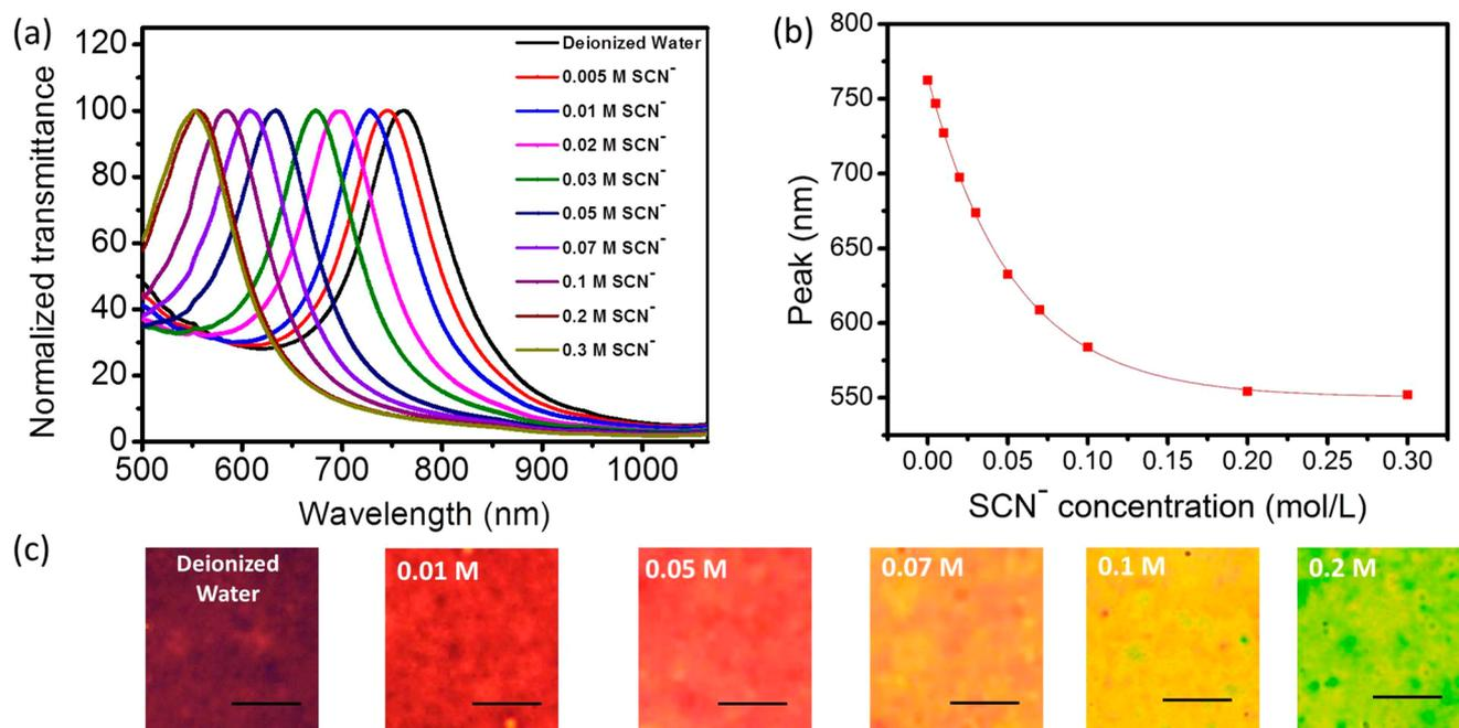
**Figure 2.** (a) Transmittance spectra of the as-prepared MIM resonator in different solutions. (b) Relation curve between the shift of the peak and the concentration of the SCN<sup>-</sup> solutions. (c) Optical photographs of the as-prepared MIM resonator in different concentrations of SCN<sup>-</sup> solutions (the bar is 10  $\mu$ m).
