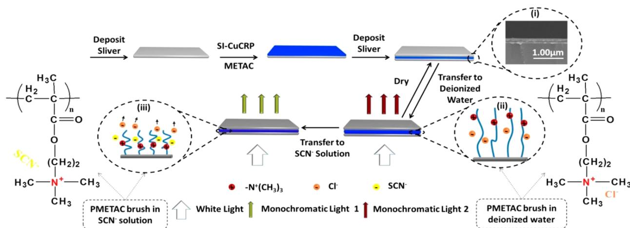
**Figure 1.** Schematic diagram of the preparation process and the detection principle of the as-prepared MIM resonator. Insets show the cross-sectional SEM image of the MIM resonator (i) and the conformation of PMETAC chain in deionized water (ii) and electrolyte solution (iii).
