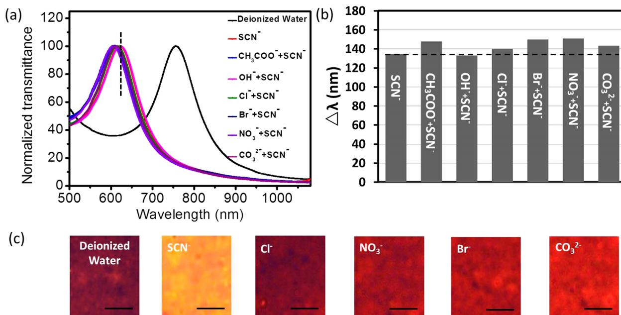
**Figure 3.** (a) Transmittance spectra of the as-prepared MIM resonator in water, SCN<sup>-</sup>, and mixtures of SCN<sup>-</sup> and disturbing anions. (b) Peak shift of the as-prepared MIM resonator for detecting SCN<sup>-</sup> in different solutions and water. (c) Photographs of the as-prepared MIM resonator in different anion solutions (the bar is 10 μm).
