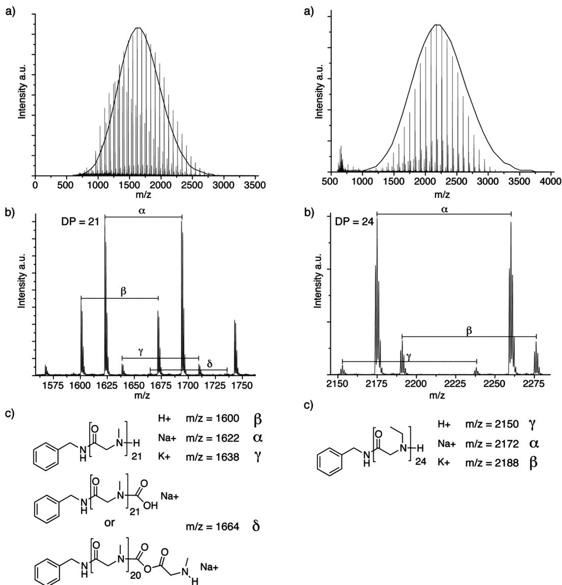
**Figure 4.** MALDI–ToF mass spectra ( $\text{H}^+$  doping, matrix DA) of (a) **P1** (left column) and **P4** (right column), with an overlay of the respective Poisson distributions (black curve) along with (b) a blown up view of section comprising most intensive signals. (c) Structures of polymers that can be assigned to the different populations.
