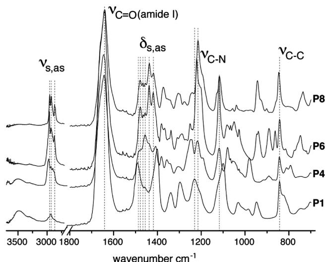
Figure 6. Comparison of IR spectra of PSar (P1), P(EtGly) (P4), P(nPrGly) (P6), and P(nBuGly) (P8). The increased intensity of the water band at around 3400 cm<sup>-1</sup> reflects the increased hydrophilicity and hygroscopic character of P1 and P4 as compared to P6 and P8.
