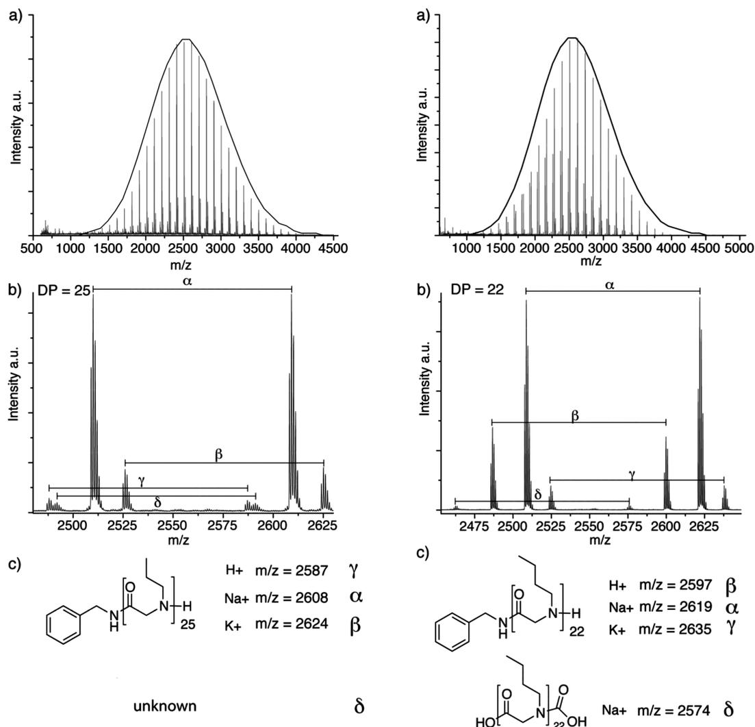
**Figure 5.** MALDI–ToF mass spectra ( $H^+$  doping, matrix DA) of (a) P6 (left column) and P8 (right column) with an overlay of the respective Poisson distributions (black curve) along with (b) a blown-up view of section comprising most intensive signals. (c) Structures of polymers that can be assigned to the different populations.
