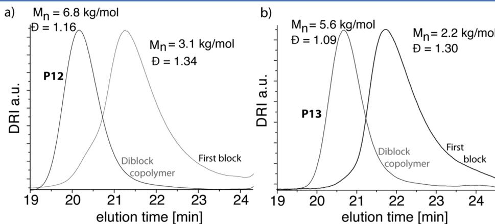
**Figure 7.** Gel permeation chromatography of the first block and final product of (a) P12 and (b) P13. The complete consumption of the first block indicates the successful preparation of amphiphilic block copolypeptide of Sar and nBuGly.
