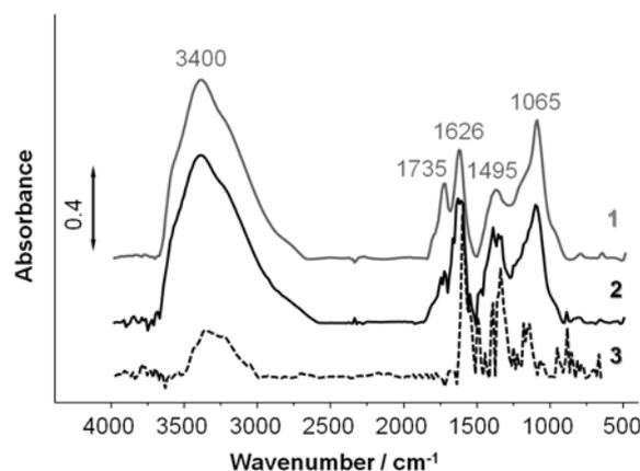
Figure 7. FT-IR spectra of GO (curve 1), MB adsorbed on GO (curve 2) and solid MB (curve 3).
