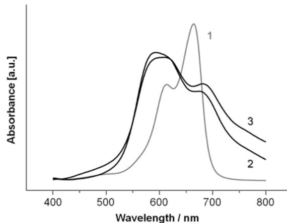
**Figure 10.** UV-Vis spectra of  $2.5 \times 10^{-5}$  M MB solution (curve 1), MB-GO nanostructure, immediately after mixing in water (curve 2, with 4x amplification), and after 24h adsorption time (curve 3, with 4x amplification).
