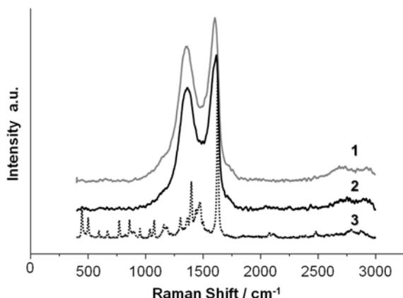
**Figure 16.** Raman spectra, excited at 532 nm of GO-T (1), MB adsorbed on GO-T (2) and solid MB (3).
