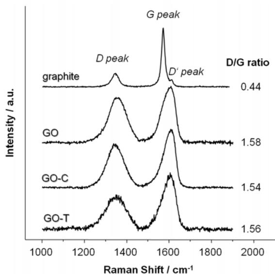
Figure 6. Comparison of Raman spectra of all graphitic derivatives.
