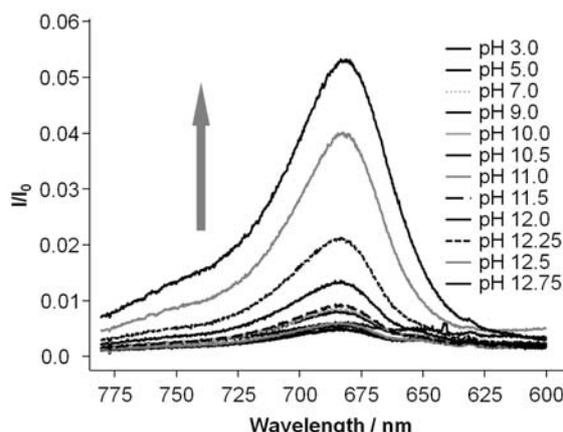
**Figure 18.** Emission spectra of aqueous solution of MB-GO composite at different pH values ( $C_{MB} = 5 \times 10^{-5}$  M,  $C_{GO} = 0.1$  g/l, adsorption time 24h, excitation wavelength 532 nm, 0.5 mW, 60x1s).
