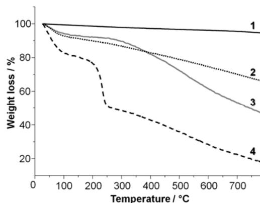
**Figure 1.** TGA of pristine graphite, PG (curve 1), chemical reduced graphite oxide, GO-C (curve 2), thermal reduced graphite oxide, GO-T (curve 3), and graphite oxide, GO (curve 4).
