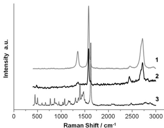
**Figure 13.** Raman spectra of graphite (curve 1), MB adsorbed on graphite (curve 2), and solid MB (curve 3) (excited at 532nm).
