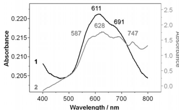
**Figure 11.** UV-Vis absorption spectra of MB-GO composites: MB-GO dispersed in water (curve 1), MB-GO solid film on quartz (curve 2) ( $c_{MB} = 5 \times 10^{-5}$  M,  $c_{GO} = 0.1$  g/l, adsorption time 24h).
