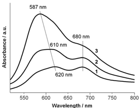
**Figure 9.** Comparison of UV-Vis spectra of MB-GO dispersions from different MB concentrations:  $10^{-5}$  M (curve 1),  $2.5 \times 10^{-5}$  M (curve 2),  $5 \times 10^{-5}$  M (curve 3) ( $c_{GO} = 0.1$  g/l, adsorption time 24h).
