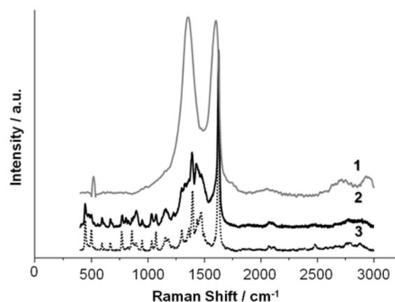
**Figure 14.** Raman spectra of GO (1), MB adsorbed on GO (2) and solid MB (3). (excited at 532nm)
