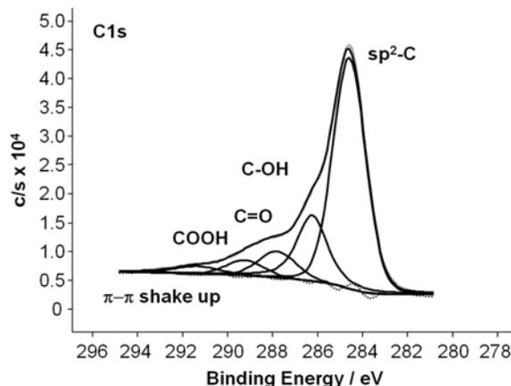
Figure 4. High resolution XPS C1s single spectrum of GO-T.
