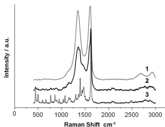
**Figure 15.** Raman spectra of GO-C (1), MB adsorbed on GO-C (2) and solid MB (3). (excited at 532nm)
