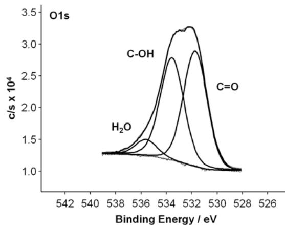
Figure 5. High resolution XPS O1s single spectrum of GO-T
