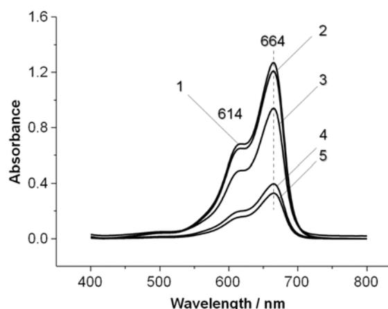
Figure 8. UV-Vis spectra of aqueous solution of MB ( $10^{-5}\text{M}$ ) (curve 1), MB adsorbed on PG (curve 2), MB adsorbed on GO-T (curve 3), MB adsorbed on GO-C (curve 4) and MB adsorbed on GO (curve 5).
