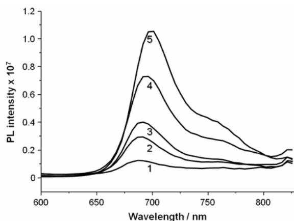
**Figure 17.** Emission spectra of aqueous solution of MB at different concentrations:  $2.5 \times 10^{-6}$  (1),  $5 \times 10^{-6}$  (2),  $10^{-5}$  (3),  $2.5 \times 10^{-5}$  (4),  $5 \times 10^{-5}$  (5), (excitation wavelength 620 nm).
