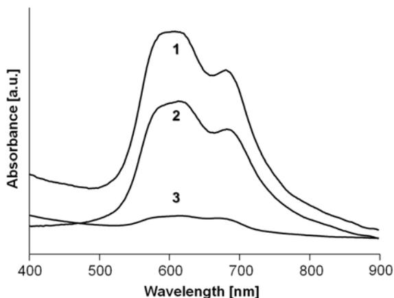
**Figure 12.** UV-Vis absorption spectra of MB-GO dispersions (curve 1), MB-GO after treatment with ultrasound (curve 2), MB solution after centrifugation (curve 3) ( $C_{MB} = 5 \times 10^{-5} M$ ,  $C_{GO} = 0.1 g/l$ ).
