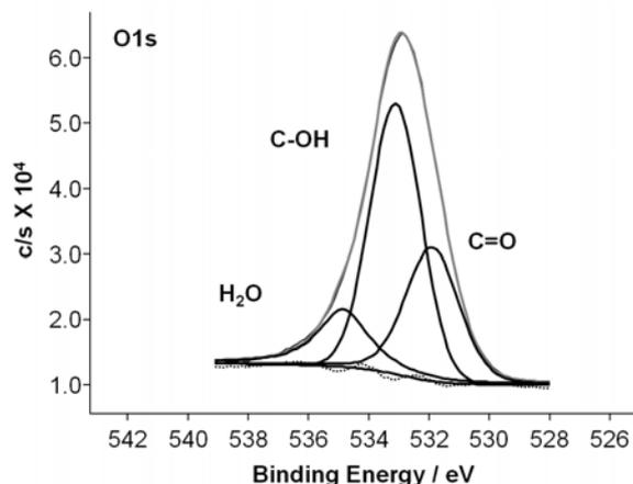
Figure 3. High resolution XPS O1s single spectrum of GO.
