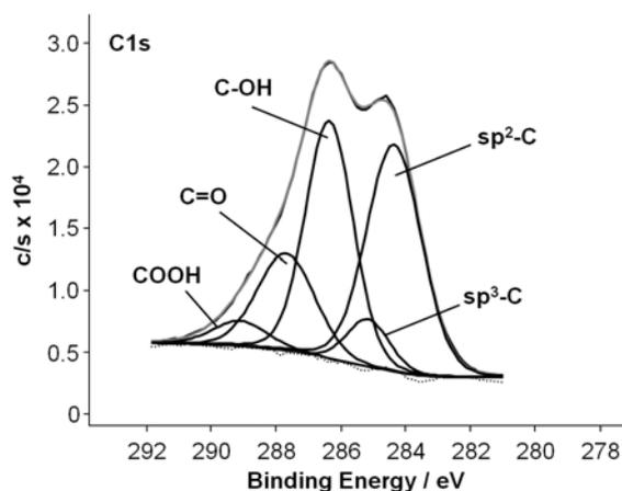
Figure 2. High resolution XPS C1s single spectrum of GO.
