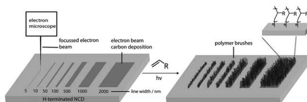
**Fig. 1** Preparation of structured polymer brushes on diamond. On the native NCD surface structures of electron beam-induced carbon deposits are created by means of a focussed electron beam. The 10  $\mu\text{m}$  long CT lines had widths of 2  $\mu\text{m}$ , 1  $\mu\text{m}$ , 500 nm, 100 nm, 50 nm, 10 nm and 5 nm. The carbon templates were amplified by the SIPGP to structured polymer brushes.
