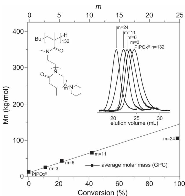
**Figure 2.** Plot of  $\bar{M}_n$  of molecular brushes using macroinitiator M<sup>II</sup> as a function of monomer conversion (2-*n*-propyl-2-oxazoline) and the degree of polymerization of side chains,  $m$ , as determined by GC. Inset: Gel permeation chromatography elugrams of the corresponding polymers.
