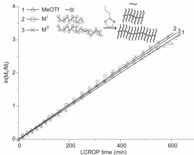
**Figure 1.** First-order kinetic plots for the grafting polymerization of 2-*n*-propyl-2-oxazoline in the presence of monofunctional MeOTf (1) and plurifunctional macroinitiators M<sup>I</sup> (2) and M<sup>II</sup> (3).
