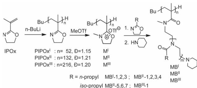
**Scheme 1.** Reaction scheme for the preparation of molecular brushes of poly(2-oxazoline)s (POx). Synthesis of the molecular brush backbone by living anionic polymerization of 2-isopropenyl-2-oxazoline (IPOx), followed by conversion to the macroinitiator and formation of side chains by living cationic ring-opening polymerization of 2-*n*-propyl (nPrOx) and 2-*iso*-propyl-2-oxazoline (iPrOx) and termination with piperidine.
