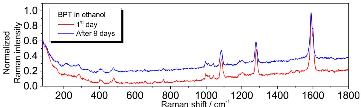
**Figure 4:** Comparison Raman spectra of averaged spectra of the first day (red line) and after 9 day (blue line) of electrochemically etched silver wires with a SAM coating of ethanol-immersed 4-biphenylthiol (BPT) with a difference spectrum of the averaged spectra as insert.
