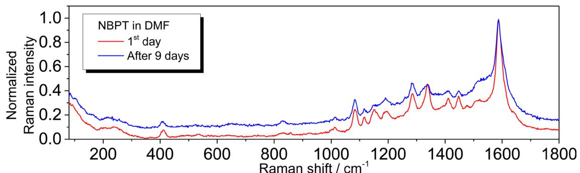
**Figure 5:** Comparison Raman spectra of averaged spectra of the first day (red line) and after 9 day (blue line) of electrochemically etched silver wires with a SAM coating of DMF-immersed 4'-nitro-4-biphenylthiol (NBPT) with a difference spectrum of the averaged spectra as an insert.
