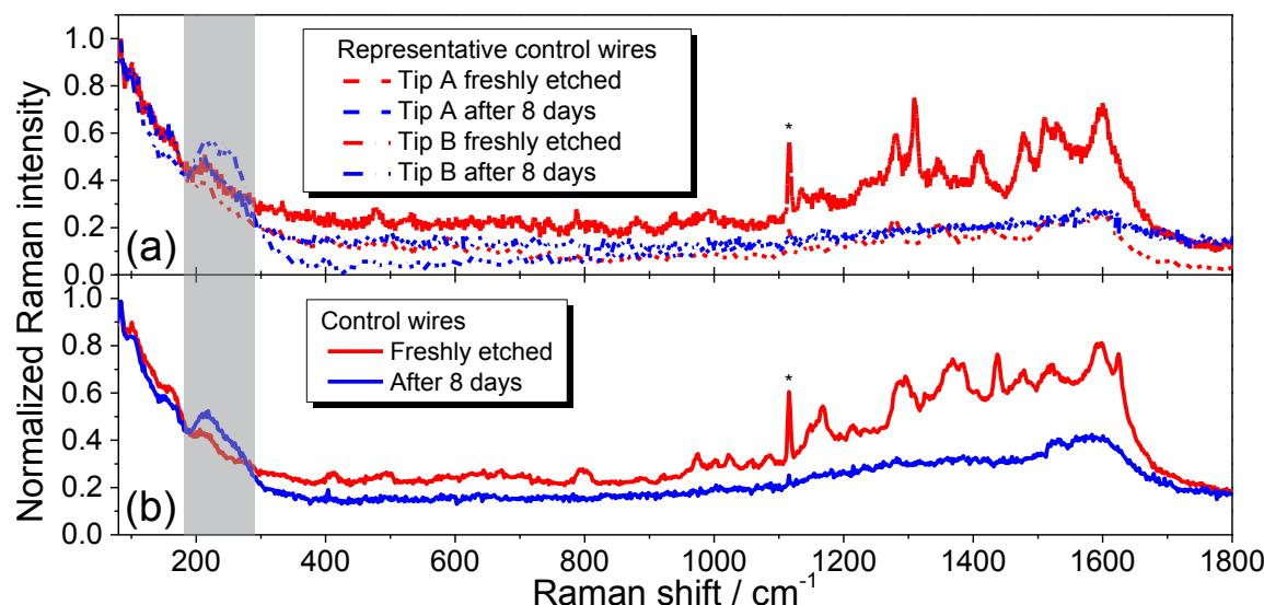
**Figure 2:** Representative Raman spectra of two freshly etched wires and wires after 8 days of aging (a) and averaged Raman spectra of all freshly etched and after 8 days control wires (b). In area in grey colour, the Raman bands can be attributed to the silver corrosion process. The asterisk indicates peak of parasitic visible light.
