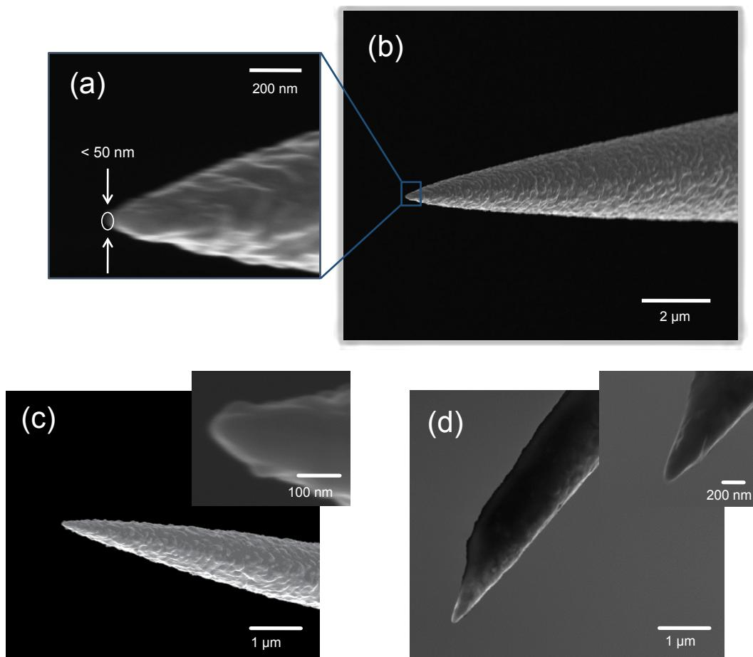
**Figure 7:** Typical SEM micrograph (b) of an electrochemically etched silver probe, (a) with enlarged tip apex, (c) a wire apex coated with a monolayer BPT (d) and NBPT – both immersed in DMF – with insets of higher magnification. From the SEM micrographs no change in surface morphology was observed.
