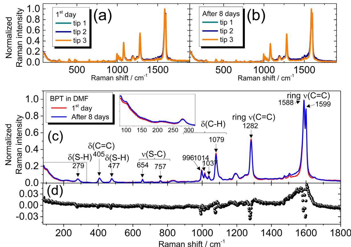
**Figure 3:** (a) Raman spectra of electrochemically etched silver wires with a SAM coating of 4-biphenylthiol (BPT) immersed in DMF. Several representative spectra of SAM protected wires measured on the first day immediately after assembly, (b) after 8 days, (c) comparison of averaged spectra of the first day (red line) and on the 8<sup>th</sup> day (blue line), (d) and difference spectrum of averaged spectra.
