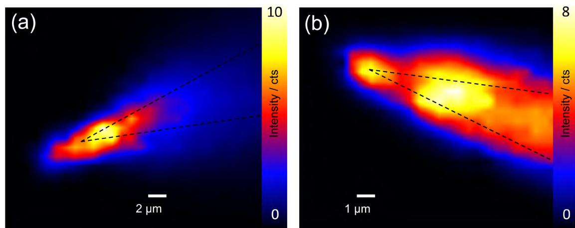
**Figure 6:** (a) Raman intensity mapping of the 1589 cm<sup>-1</sup> band of the electrochemically etched wire apex with SAM coating of BPT, (b).and NBPT
