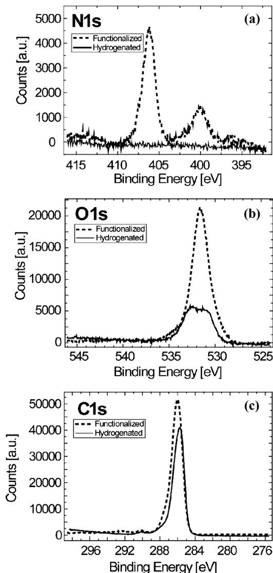
**Figure 2.** (a) N1s XPS spectra of a NB-functionalized diamond surface as compared to a reference sample of hydrogenated UNCD. Details of the O1s (b) and C1s (c) core level spectra of the same two samples.
