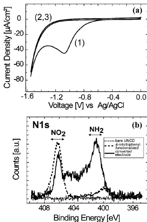
**Figure 6.** (a) Cyclic voltammogram of an NB-functionalized UNCD electrode recorded in 100 mM potassium chloride aqueous electrolyte solutions. The first scan (1) shows an irreversible wave, peaking at  $-1.08$  V vs Ag/AgCl, corresponding to the reduction of the residual nitro groups. (b) N1s core level XPS spectra of the NB-functionalized electrode before and after the electrochemical reduction. For comparison, a hydrogenated reference sample (bare UNCD) was recorded (dotted line).
