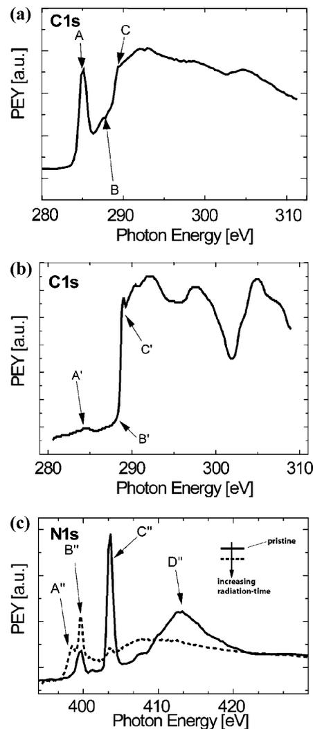
**Figure 5.** (a) Photon yield C1s NEXAFS absorption spectra of a biphenyl grafted UNCD sample. An intense  $\text{C}1\text{s} \rightarrow \pi^*$  resonances, feature A, occurs in the absorption spectra, originating from the  $\pi$ -bonded carbon atoms within the phenyl ring. (b) NEXAFS spectra of a hydrogenated UNCD sample. (c) NEXAFS spectra recorded at the N1s edge. The following subsequently recorded spectra show a radiation induced peak change of the  $\sigma^*$  and  $\pi^*$  resonances.
