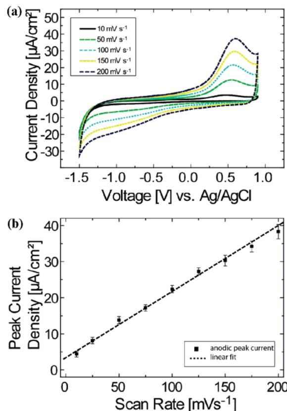
**Figure 7.** (a) Cyclic voltammograms of a reduced, NB-functionalized doped UNCD diamond electrode in 100 mM potassium chloride aqueous solution at various scan rates (10 to  $200 \text{ mV s}^{-1}$ ). (b) Plot of the maximum anodic peak current density versus the scan rate.
