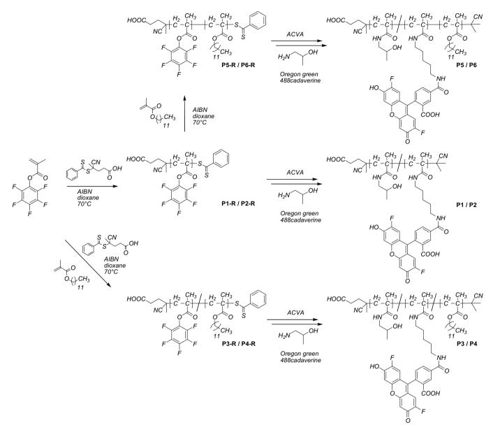
Scheme 1. Synthetic pathway to fluorescently labelled homopolymers, random copolymers and block copolymers based on pHPMA using the active ester approach.
