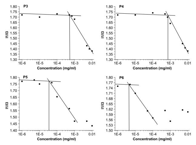
Fig. 1. The cmc estimation of random copolymers P3, P4 and block copolymers P5, P6 by pyrene fluorescence spectroscopy in isotonic solution at pH 7.
