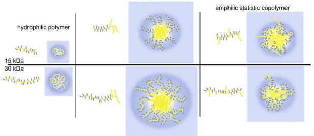
Fig. 2. Schematic sketch of self-assembled polymeric structures in aqueous solution (blue parts: hydrophilic, yellow parts: hydrophobic). Homopolymers are present as unimers (left), block copolymers from polymer micelles or micelle-like core-shell aggregates (center) while random copolymers can form less stable aggregates through intra- and interchain interactions.
