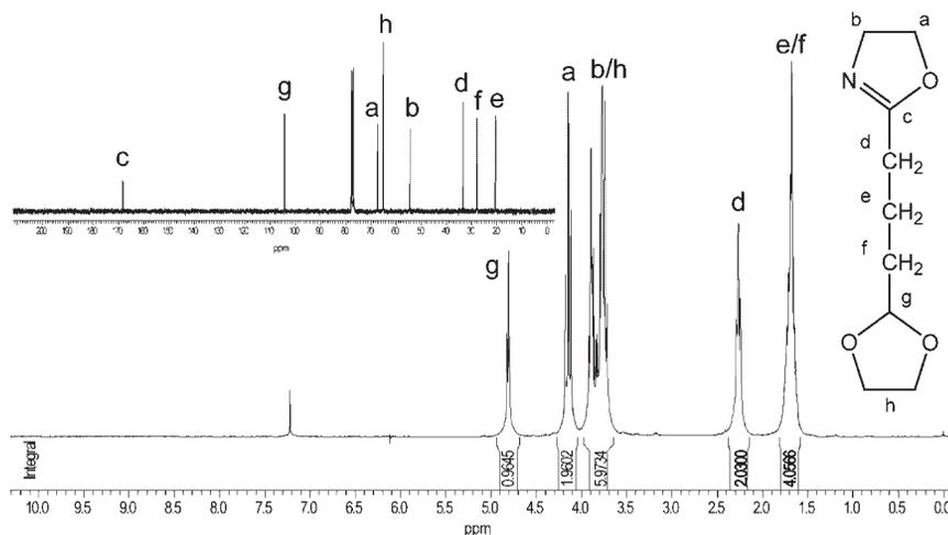
Figure 1.  $^1\text{H}$  and  $^{13}\text{C}$  NMR spectra (insert) of **DPOx**. All signals could be assigned; residual side products were not detected after purification. Signals h and g are characteristic for the 1,3-dioxolan ring (for details see Experimental Part).
