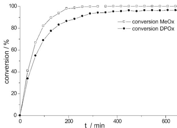
Figure 2. Conversion of **MeOx** and **DPOx** with time as monitored by on-line GC sampling. Conversion of **DPOx** appears to be slightly slower; however, the rate of conversion is comparable for both monomers. (Note: Final conversion is <100% due to contamination by the multiple sample collection.)
