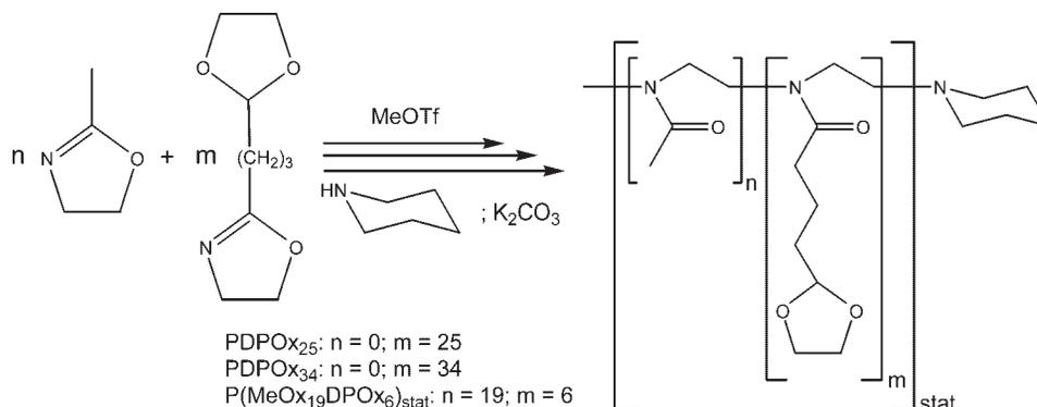
Scheme 2. One-pot preparation of poly(2-oxazoline)s with different amounts of protected side chain aldehyde.
