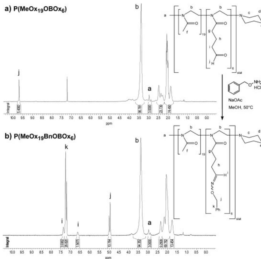
Figure 4.  $^1\text{H}$  NMR spectra and reaction scheme of the chemoselective ligation of aldehyde-functionalized poly(2-oxazoline) with *O*-benzylhydroxylamine hydrochloride. The final product can have the *cis* and *trans* configuration.
