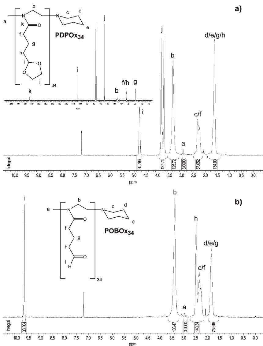
Figure 3. <sup>1</sup>H NMR spectra of (a) PDPOX<sub>34</sub>. Acid hydrolysis with TFA yields quantitative conversion into the aldehyde function of POBOX<sub>34</sub> (b).
