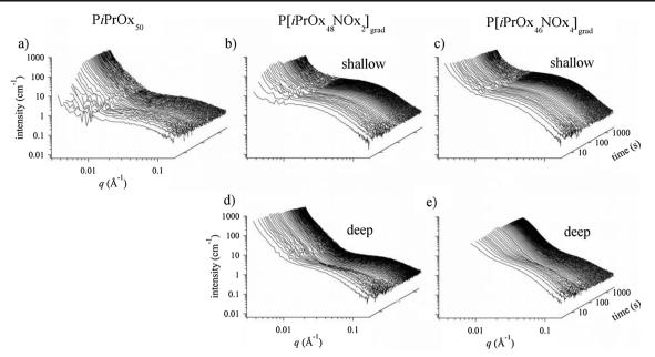
**Fig. 2** SANS curves taken during the temperature jumps. **a**  $PiPrOx_{50}$ ,  $T_{Target}=39.8$  °C. **b**, **d**  $P[iPrOx_{48}NOx_2]_{grad}$ ,  $T_{Target}=27.0$  °C (**b**) and 30.0 °C (**d**). **c**, **e**  $P[iPrOx_{46}NOx_4]_{grad}$ ,  $T_{Target}=22.2$  °C (**c**) and 27.3 °C (**e**)
