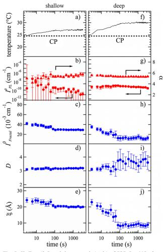
**Fig. 5** Shallow (*left*) and deep quench (*right*) of  $P[iPrOx_{48}NOx_2]_{grad}$ . Same notations and symbols as in Fig. 4. The *arrows* in (**b**, **g**) indicate the axis used for the respective values. For better visibility, data points at later times are omitted
