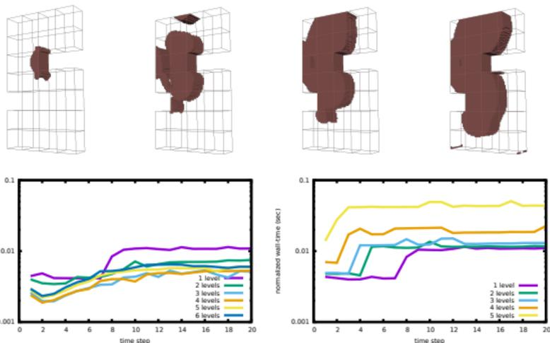
Normalized wall-time per time step: TNNMG (left) vs. predictor-corrector (right)
