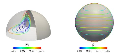
Figure 5.4: Streamlines of the inner velocity  $\mathbf{V}_2$  (left) and streamlines of the surface fluid viewed from top (right) for  $\epsilon = 0.01$ .
