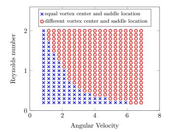
Figure 3.12: Reynolds number against angular velocity phase diagram. Here it is assumed that the vortex is placed off the Gaussian saddle if  $||(m_x, m_y)^T - (x, y)^T|| \ge 0.1$  (red circles). Blue crosses indicate high geometric influences through vortex trapping.
