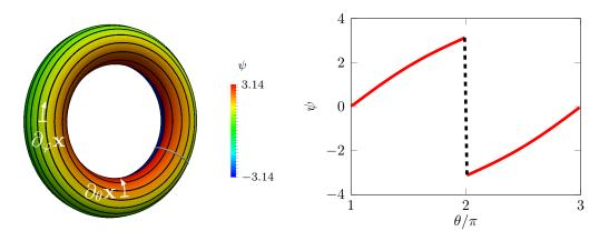
Figure 3.2: Left: Streamlines and values of the discontinuous stream function  $\psi$  to represent the velocity field  $\hat{\mathbf{v}} = \partial_{\varphi} \boldsymbol{x}$  on the torus and the two basis vectors  $\partial_{\varphi} \boldsymbol{x}$  and  $\partial_{\theta} \boldsymbol{x}$ . Right: Plot of the stream function values over the gray contour line in the left figure.
