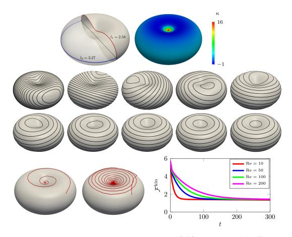
Figure 3.8: Top: Distances on the biconcave shape (left) together with the Gaussian curvature (right). Middle: Streamlines at times t = 0, 7, 14, 21, 28, 35, 42, 49, 56 and 200 (left to right, top to bottom) for the rotating flow. Results are shown for Re = 10. Bottom: Two examples for the vortex trajectories for Re = 10 (left) and Re = 100 (center) and kinetic energy  $\mathcal{F}^{kin}$  against time t for various Reynolds numbers Re (right).
