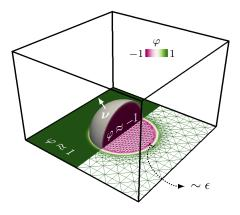
Figure 5.2: Implicit description of the computational domain  $\Omega = \Omega_1 \cup S \cup \Omega_2$  using a phase field function  $\varphi$ , together with the adaptively refined mesh. Note that the height of the bounding box is not proportional to the rest of the domain due to visual clarity.
