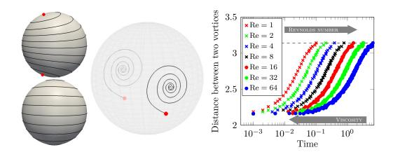
Figure 3.3: Left: Streamlines for the initial condition (top) and the reached steady state solution (bottom) for Re = 1. Center: Vortex trajectories on the sphere for Re = 100. The red points (left and center) indicate the respective initial positions of the vortices. Right: Geodesic distance between the two vortices over time for various Reynolds numbers. The gray arrows indicate increasing Reynolds number and viscosity.
