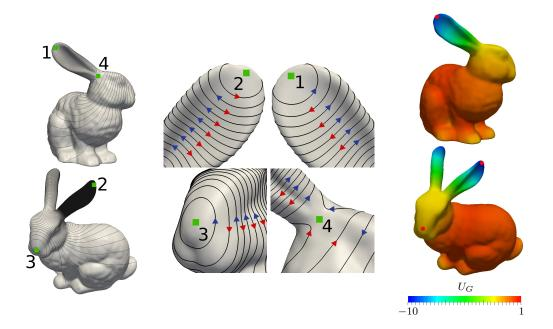
Figure 3.6: Left: Streamlines of the flow field on the Stanford bunny with the green marked positions of the different defects. Numbers 1 to 3 indicate vortices (+1 defects) and number 4 indicates a saddle point (-1 defect). Center: Identified defects with rescaled streamlines and different flow directions (red and blue arrows) according to different realizations of the noise initial condition. Right: Geometric potential  $U_G$  with identified local minima (red points).
