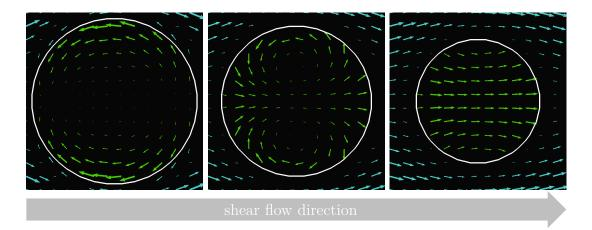
Figure 5.3: Two dimensional velocity (projected to the plane and rescaled for visualization) of the sliced  $L_d$  vesicle at height levels z = 0.3, 0.5, 0.7 (from left to right) for  $\epsilon = 0.01$ . The green arrows indicate the inner velocity  $\mathbf{V}_2$  and the blue arrows indicate the outer velocity  $\mathbf{V}_1$ . Shear direction is from left to right.
