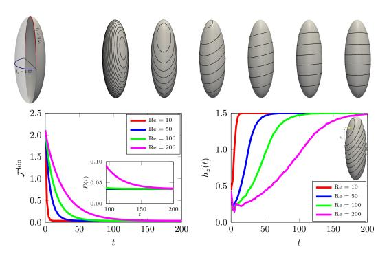
Figure 3.7: Top: Distances on the ellipsoid (left) together with the streamlines at times t = 0, 4, 8, 12, 16 and 20 for the rotating flow (left to right). Results are shown for Re = 10. Bottom: Kinetic energy  $\mathcal{F}^{\text{kin}}$  against time t (left) and the height for the upper vortex  $h_z$  against time t for various Reynolds numbers Re.
