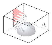
Figure 5.1: Schematic computational domain  $\Omega_1$ ,  $\Omega_2$  and S to consider the experimental setting in [VMV07, HSWKG13]. The red arrows indicate the shear flow through the domain and  $\dot{\gamma}$  denotes the shear rate. At the bottom the vesicle is adhered to a solid wall.
