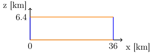
Figure 12: Domain and boundary for the cold bubble down blast benchmark. The orange line represents a rigid boundary, i.e. \mathbf{u} = \mathbf{w} = 0 with zero normal pressure gradient. The blue lines represent the periodic boundary.
