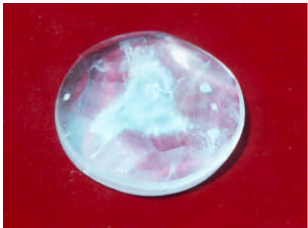
Fig. 4: A typical crystal grown by the flux pulling technique, here the inclusions that are three-fold axisymmetrically distributed in the central part can be seen
