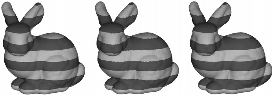
**Figure 12.** Image denoising with level-set representation of the surface. From left to right: original image, noisy image, image after 5 timesteps.  $[0, 4] \times [0, 4] \times [0, 4]$  grid with 192,000 grid points, grid size  $h = 0.039$  at the surface, and timestep  $\Delta t = 0.001$ .
