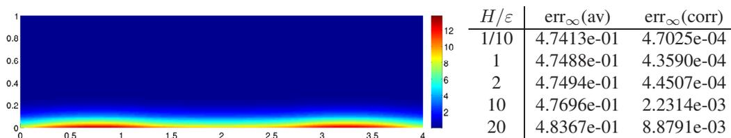
**Fig. 1:** Left: Solution at  $t_e = 100\varepsilon$ . Right: errors in simply averaged and defect corrected solution.
