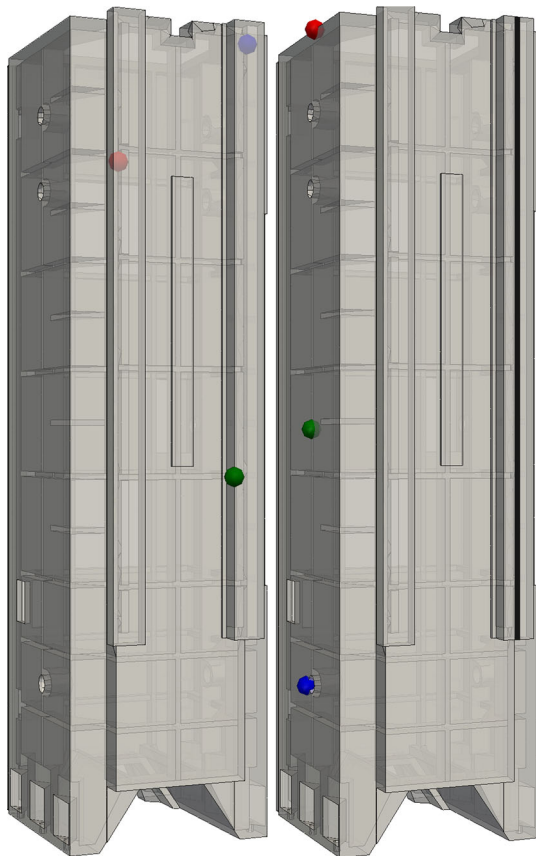
Fig. 3 Machine stand with reference points 1–6. The left figure shows the reference points 1–3 in the colors red, green and blue, respectively, whereas the right figure shows the reference points 4–6 in the colors red, green and blue, respectively (color figure online)
