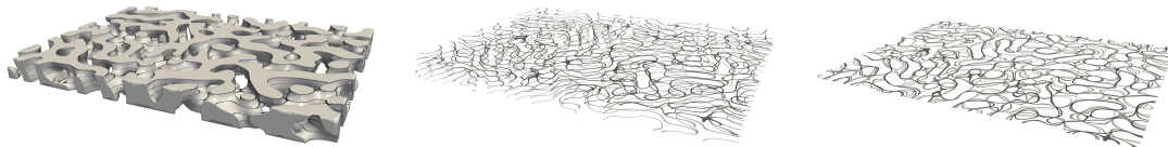
Figure 1. Typical structure within the large-time regime, visualized as \phi = 1 in \Omega , \phi = 0.5 at z = 0.01, 0.13, 0.25, 0.37, 0.49 and \phi = 0.5 at z = 0.01, 0.13, 0.25, 0.37, 0.49 projected to z = 0 , from left to right. The boundary conditions are \mathbf{n} \cdot \nabla \phi = \mathbf{n} \cdot \nabla \mu = 0 on \partial\Omega . The corresponding videos of the coarsening process are provided in SI as Videos S5–S7.
