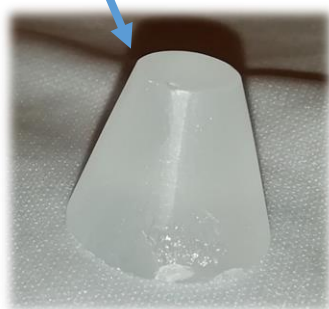
1 st ingot of the \text{Cs}_2\text{ZrCl}_6 crystal
