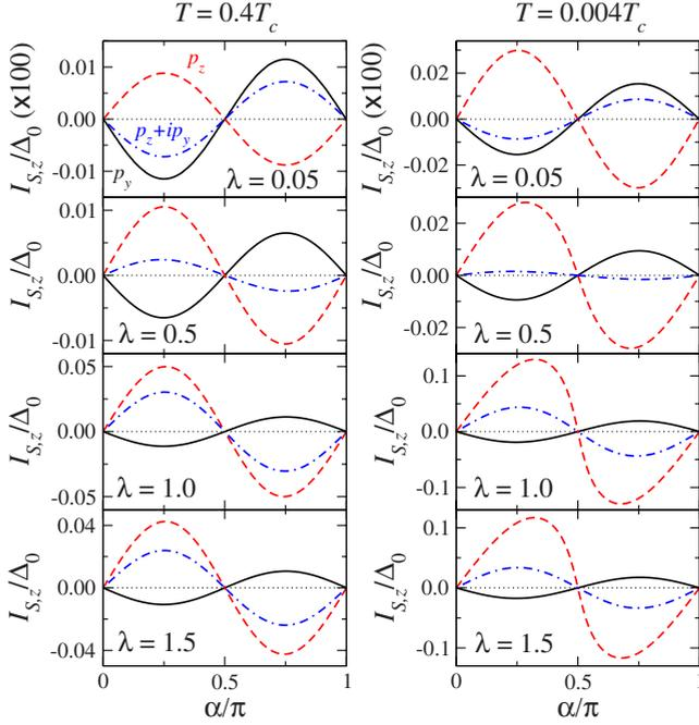
FIG. 3. (Color online) Spin current as a function of the angle  $\alpha$  for the  $p_y$  (black solid curve),  $p_z$  (red dashed curve), and  $p_z + ip_y$ -wave (blue dot-dash curve) TSCs for various values of the exchange-splitting  $\lambda$ . The left column shows the spin currents at  $T = 0.4T_c$  while the right column shows the spin currents for  $T = 0.004T_c$ .
