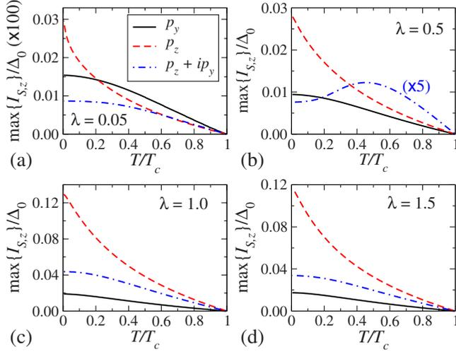
FIG. 6. (Color online) The maximum value of the spin current obtained by varying  $\alpha$  for (a)  $\lambda=0.05$ , (b)  $\lambda=0.5$ , (c)  $\lambda=1.0$  and (d)  $\lambda=1.5$ . The curves in panels (b)–(d) have the same meaning as those in panel (a); note that the  $p_z+ip_y$  curve is multiplied by 5 in (b) for clarity.
