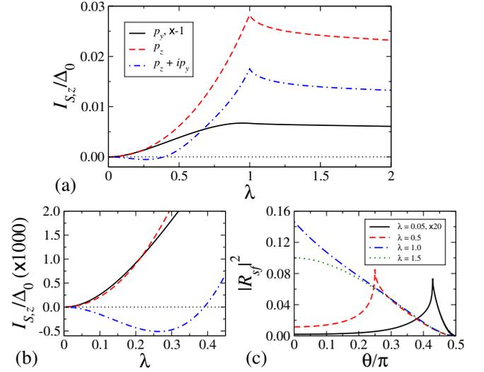
FIG. 5. (Color online) (a) Spin current as a function of the ratio  $\lambda = g\mu_B M/E_F$ . Note that the current for the  $p_z+ip_y$ -wave TSC changes sign at  $\lambda \approx 0.4$ . (b) Spin current at low  $\lambda$ . Curves have identical meaning as in panel (a). In both (a) and (b) we set  $\alpha = 0.1\pi$  and  $T = 0.4T_c$ . (c)  $T > T_c$  normal state spin-slip reflection probability as a function of the incident quasiparticle angle  $\theta$ .
