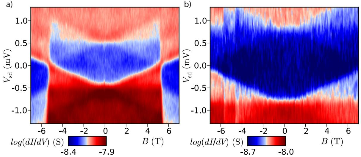
Fig.S. 2: Experimental differential conductance as a function of magnetic field for a fixed gate voltage  $V_g < V_g^D$  ( $n_{C_{60}} = 1$ ) for **(a)**  $J = -0.3$  meV (second run) and **(b)**  $J = -0.4$  meV (first run).
