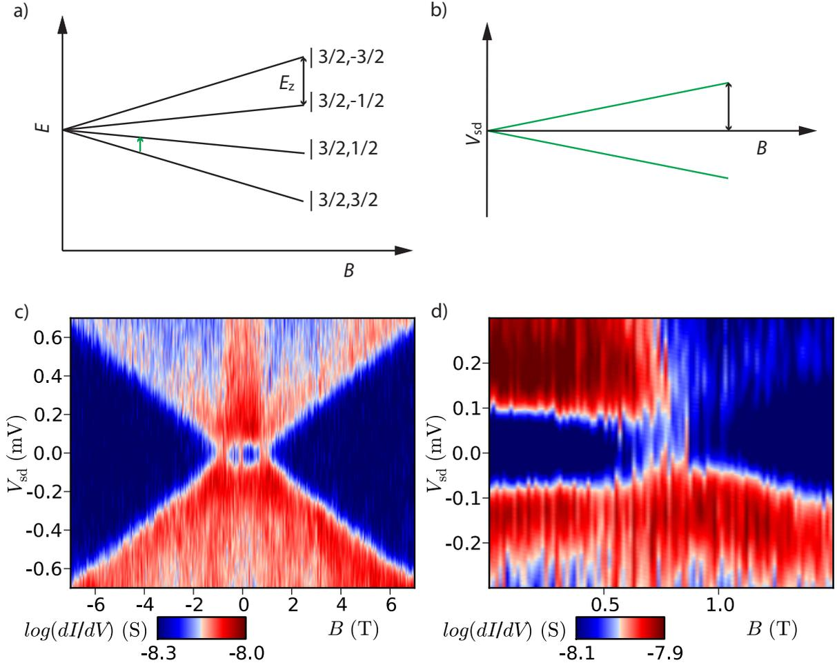
Fig.S. 3: **(a)** Zeeman diagram of the multiplet  $S = 3/2$  for  $\text{N@C}_{60}^{2-}$  ( $n_{\text{C}_{60}} = 2$ ). **(b)** Schematic showing the expected cotunneling steps deduced from the Zeeman diagram. **(c)** and **(d)**  $dI/dV$  measurements as a function of magnetic field for a fixed gate voltage.
