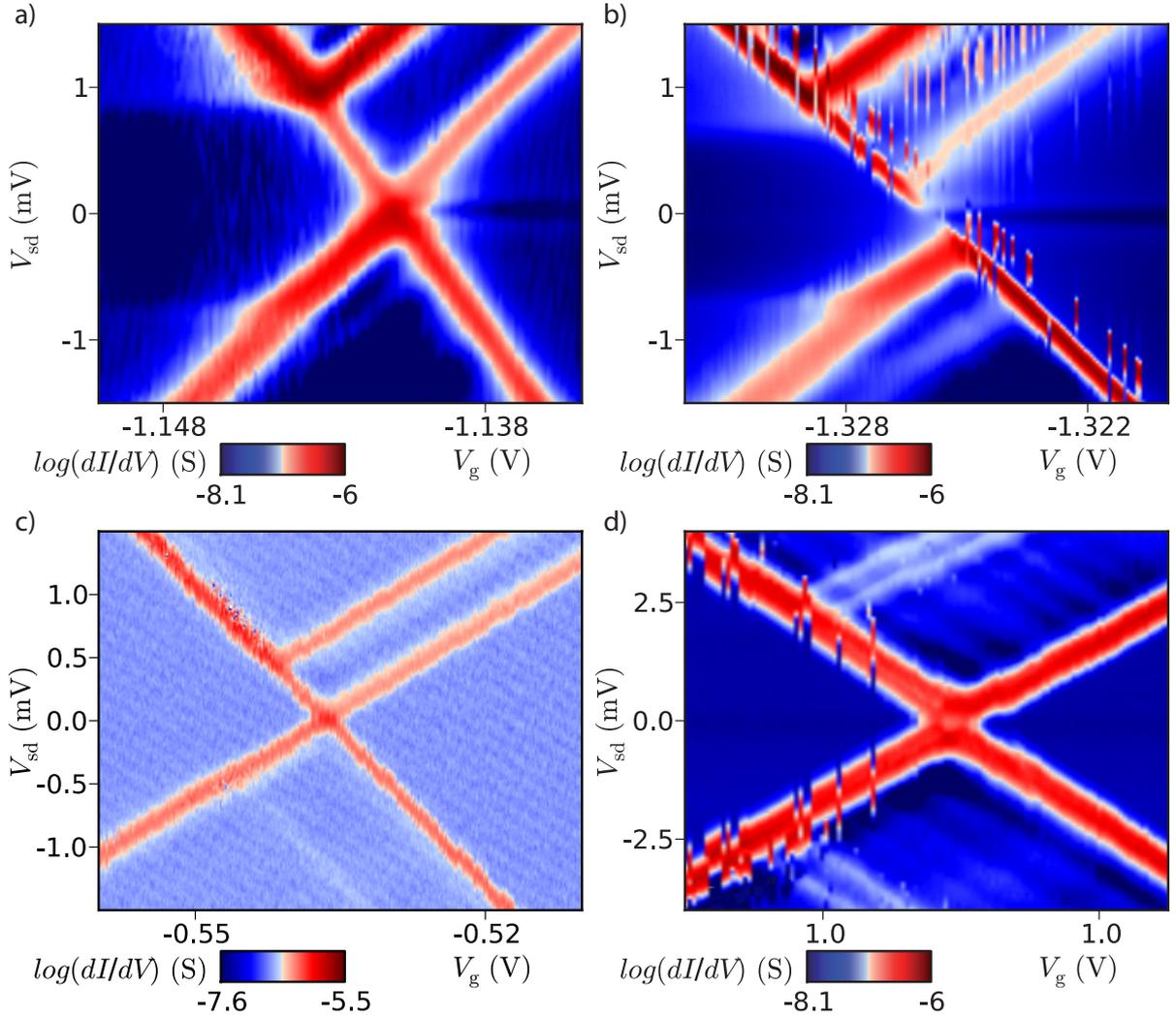
Fig.S. 1: Color scale plot of the differential conductance  $dI/dV$  as a function of bias voltage  $V_{sd}$  and gate voltage  $V_g$  : **a)** first run of measurements. **b)** second run of measurements. **c)** and **d)** other  $N@C_{60}$  SMT's in the weak coupling regime.
