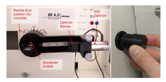
${\bf Abb.\ 2:}\ {\bf Aufbau}\ {\bf des}\ {\bf Experimentierraums}\ {\bf mit}\ {\bf Goniometer}\ {\bf und}\ {\bf Einsetzen}\ {\bf der}\ {\bf Kollimatorblende},\ {\bf Quelle:}\ {\bf PHYWE}.$
