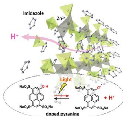
Figure. Schematic illustration of H + switching by light irradiation in glassy CP: [Zn(H 2 PO 4 )(HPO 4 )] [Imidazole] with doped pyranine.
