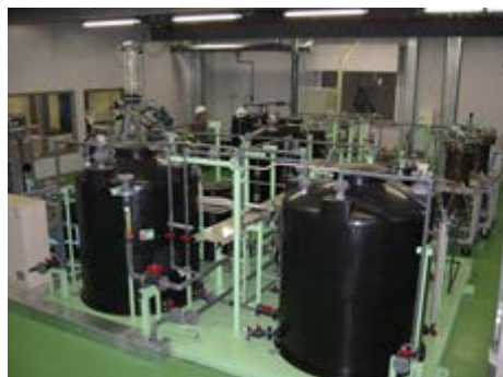
Pilot plant of lithium recovery from seawater(left) and benchmark plant of lithium recovery from salt lake brine (right)
